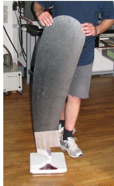
Figure 2. Horn ridge fabricated by the hybrid Al-CFRP technology.
