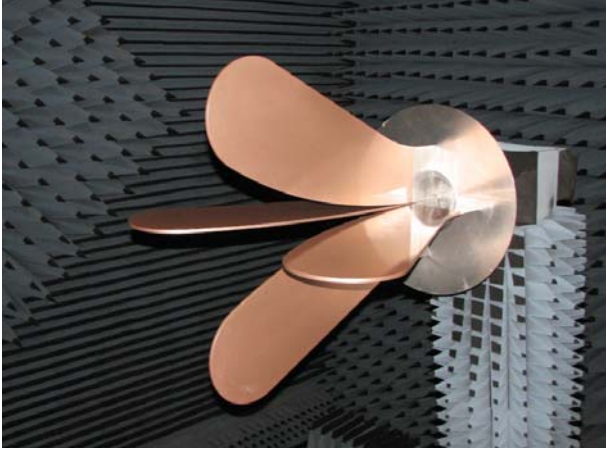
Figure 3. Manufactured hybrid Al-CFRP quad-ridge horn during radiation measurements at the DTU-ESA Facility.
