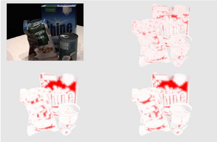
Figure 11.9: Example of a scene with missing texture compared from reference to MVS reconstruction ( R to M ). Top left is an example image. Top right is error of [33]. Bottom is reconstructions from [17] – left is multi-view and right is two-view. The colour white to red shows the error, with red having error larger than 1 cm and white points having no error.
