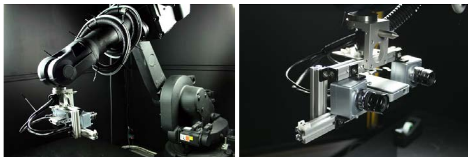
Figure 11.3: Left: Six-axis industrial robot. Right: Stereo cameras mounted on the robot arm together with a projector for structured light scanning.
