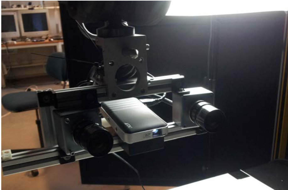
Figure 4.2: Two Point Grey Scorpion cameras and an Acer C20 mini projector mounted on the robot arm.
