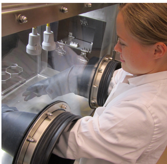
Figure 4. One of the visiting scientists is learning how to use a class III biosafety cabinet during the study visit at SVA. Photo provided by SVA.
