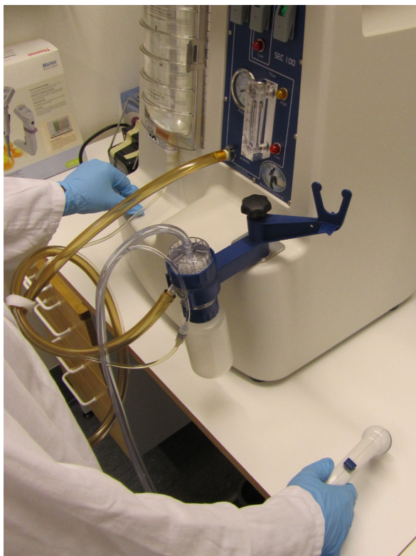
Figure 8. The MVac System sampling device uses a liquid to facilitate the extraction of microbes from a surface. The liquid is sprayed onto the surface and the extract is collected by the machine using a vacuum. Photo provided by SVA.
