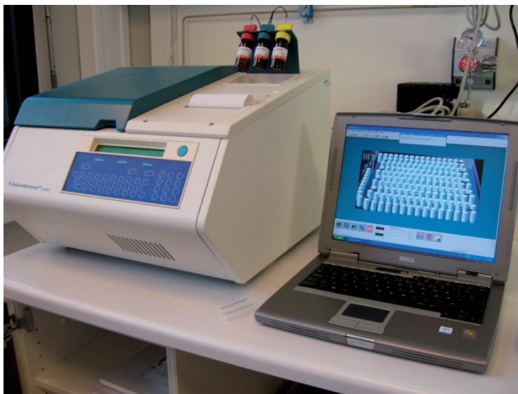
Figure 5: Example of commercial available luminometer – Celsis Advance Coupe luminometer and Advance software (Celsis Advance.im version 3). Photo: Ó.K. Vang.
