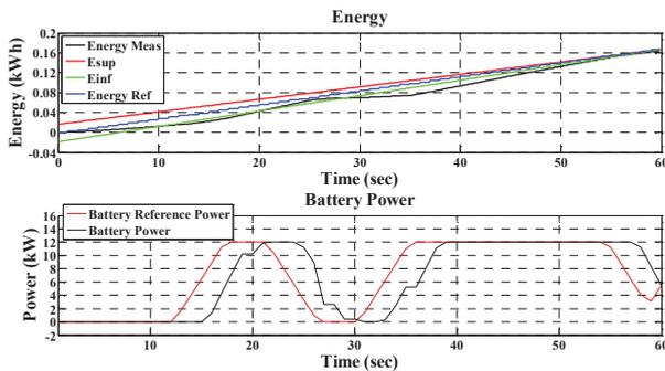
Figure 10. Energy profiles and battery power details.
