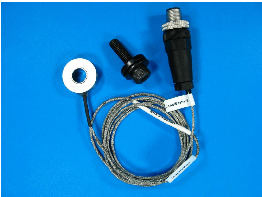
Fig. 4– LOAD WASHER LCMWD-20KN from OMEGA adopted to measure the compressive load on the bolt connecting the two shells of the TE. The load cell is mounted by means of a proper designed plate through the drilled holes in the sandwich panel. The load washer is connected to a 2,5 mm diameter string fixed through a plate to the lower panel. Any adjustment in the alignment is allowed thanks to the spherical washer set – “IGUS washer”, which provide a proper load distribution on the load cell. The initial tension on the string (compression on the load cell) is adjusted by screwing the fitting button on top (not showed in figure), in order to have a stiff configuration.
