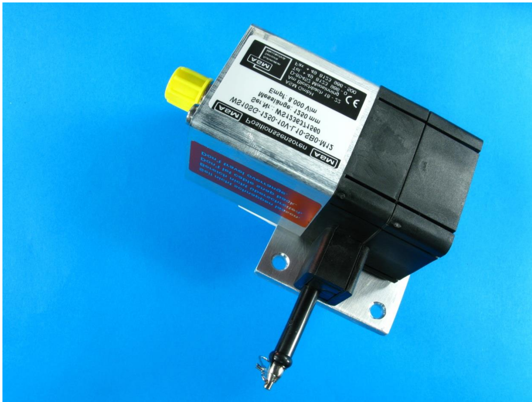
Fig. 3 – POSIWIRE WS10SG string pot from ASM, which was used in the test to measure the relative displacement between the shells in the defined points. In the picture can be noticed the connection plate then screwed to the laminate.
