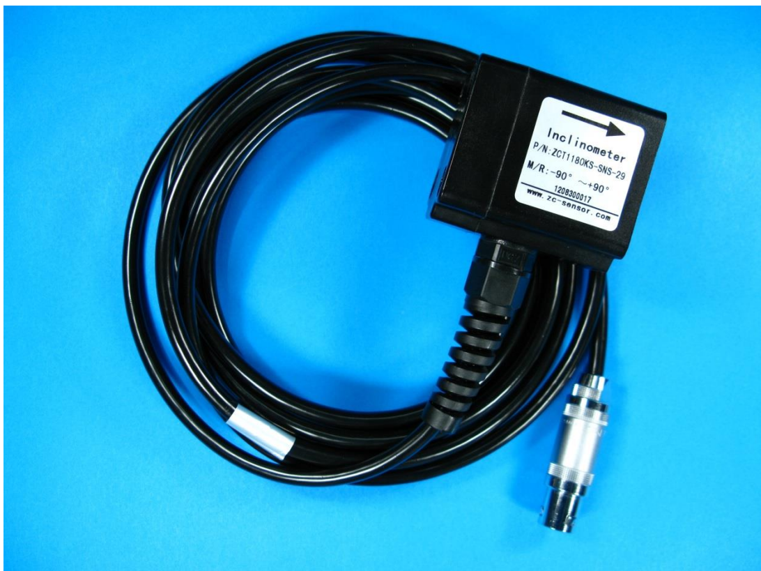
Fig. 6 – 1-axis Inclionometer sensor ZCT1180KS-SNS-29 by ZC Tech. The measuring range goes from -45^{\circ} ( -90^{\circ} ) to 135^{\circ} ( 90^{\circ} ) and the analog voltage output vary from 0,5V to 4,5V.
