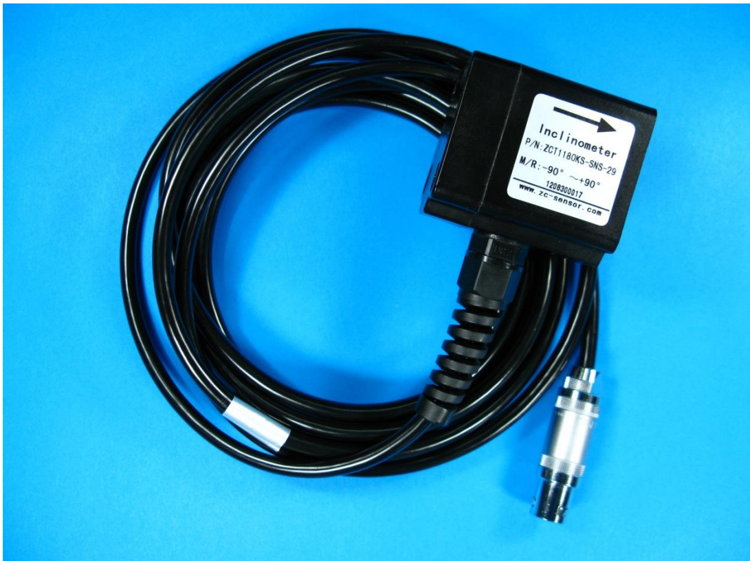
Fig. 6 – 1-axis Inclinometer sensor ZCT1180KS-SNS-29 by ZC Tech. The measuring range goes from -45^{\circ} ( -90^{\circ} ) to 135^{\circ} ( 90^{\circ} ) and the analog voltage output vary from 0,5V to 4,5V.
