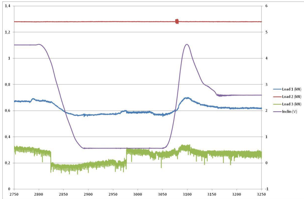
Fig. 48 - Detail from test 4 showing the blade at position 90° and changing blade pitch from 90 deg to 0 deg and then back again
