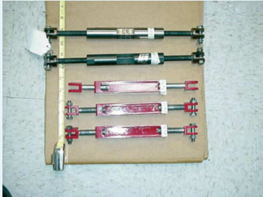
Two Alaska Airlines-fabricated restraining fixtures and three Boeing manufactured fixtures
