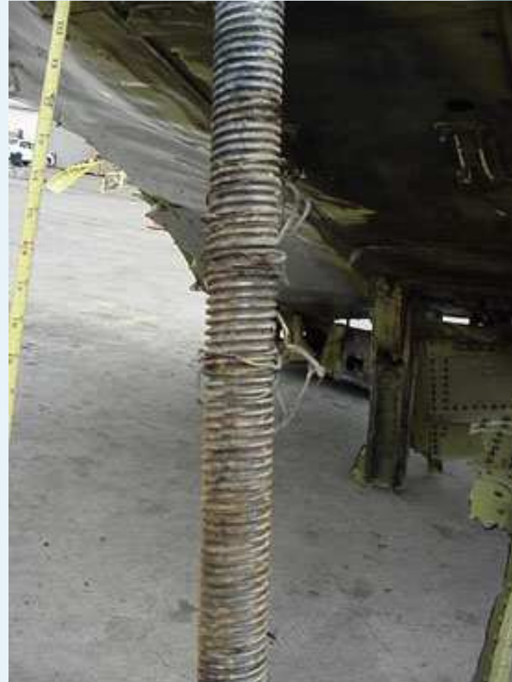
Jackscrew from horizontal stabilizer of Alaska Airlines flight 261, recovered from the wreckage
