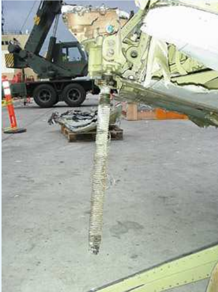
Jackscrew from horizontal stabilizer of Alaska Airlines flight 261, recovered from the wreckage
