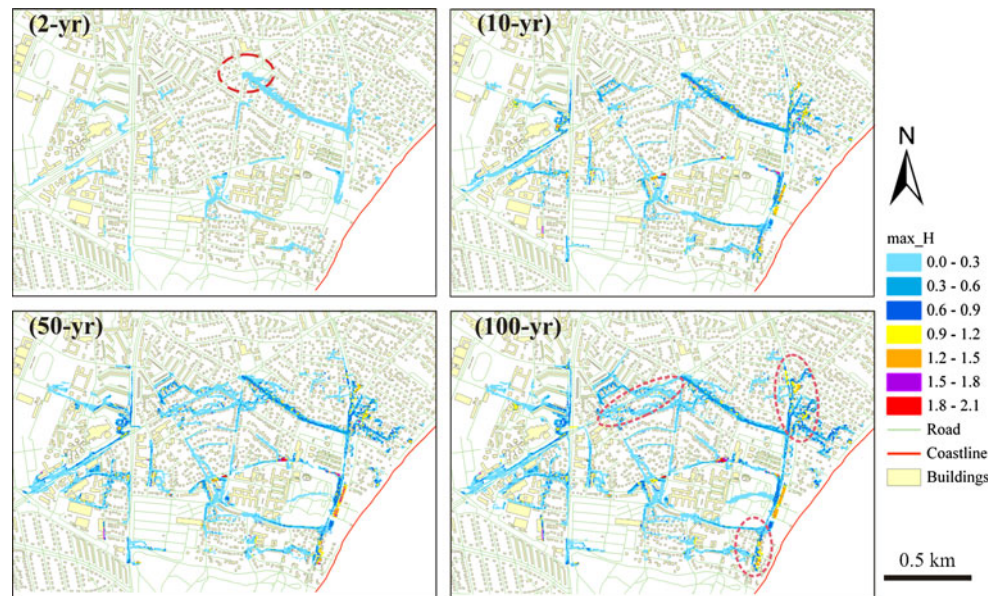
Fig. 4 Simulation of inundated extent and depth using Mike Urban and Mike Flood software package
