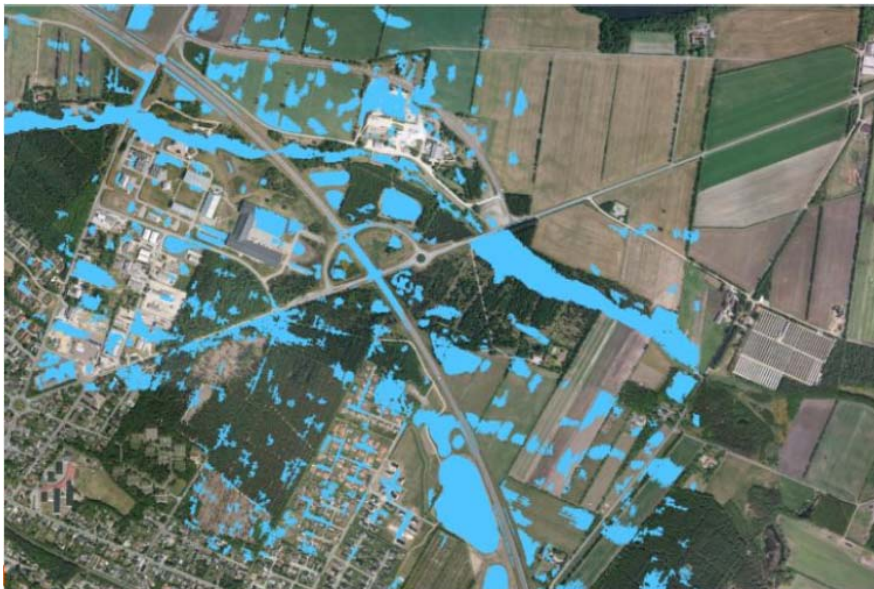
Figure 5-3 Example of a “blue spot” screening exercise of an area of potential flooding.
