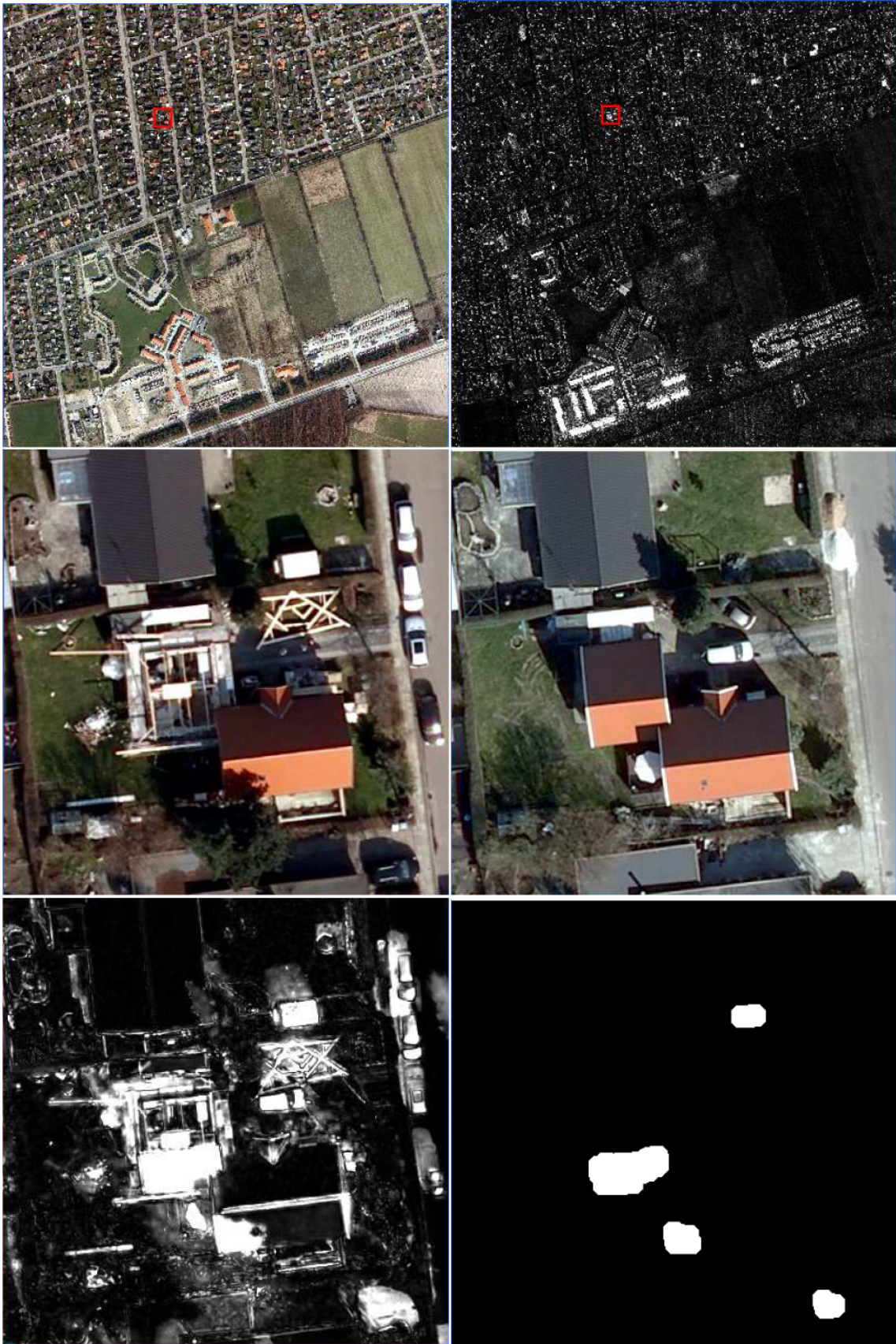
Figure 10: Example 8 for area from 6168_726. Changes between years 2007 and 2009. UL: The 2007 scene. UR: Change image. ML: Zoomed area from the 2007 scene. MR: Zoomed area from the 2009 scene. LL: Change image. LR: Significant change image.
