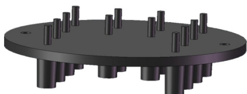
Figure 158: CAD drawing (a) and photo (b) of male luer fitting ports with external fluidic connector micro milled in Polycarbonate.
