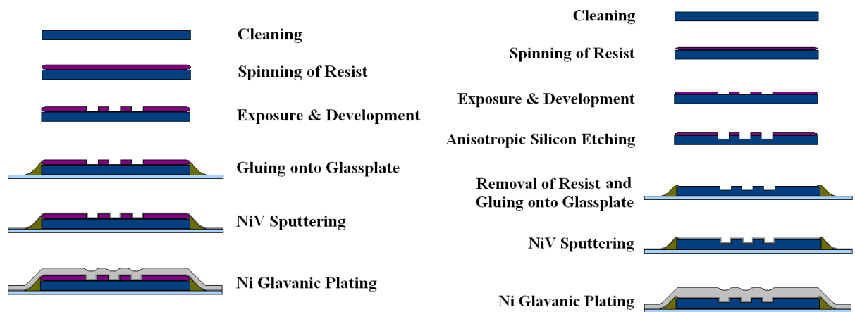
Figure 33: Cross-sectional sketch of the fabrication scheme used to fabricate master based on structured resist on silicon (upper left) and structured silicon (upper right). Separation and cutting of the resulting nickel shim follows the same scheme (left).
