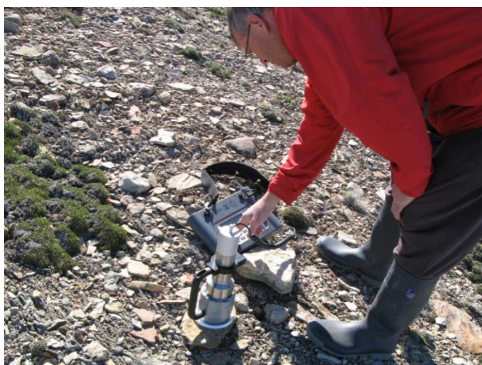
Figure 14. Portable gamma spectrometer for field measurement of ^{241}\text{Am} with detector placed on ground.
