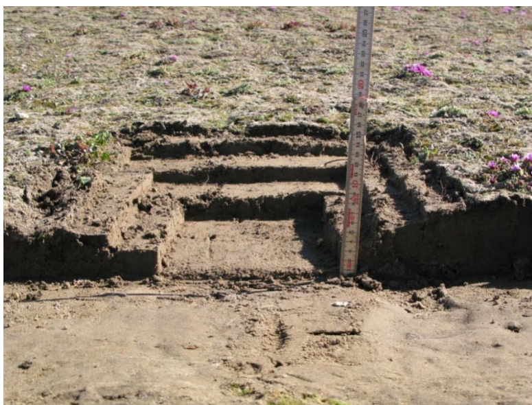
Figure 10. Sampling of soil for depth distribution 0-13 cm, sample no. 2008-4031/39, 11-Jul-2008.
