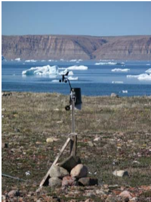
Figure 2. Weather-station sensors at Narsaarsuk recording wind speed, wind direction, temperature and precipitation.
