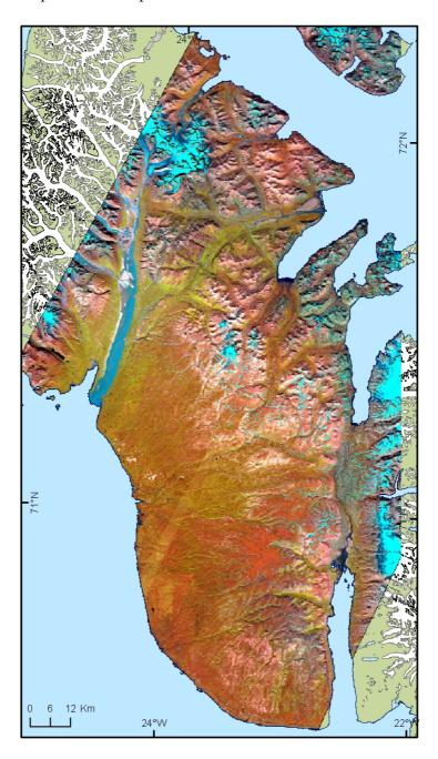
The image is a false colour composite of the shortwave infrared, the infrared and the green band (7, 4 and 3) in the red, green and blue colour channel, respectively. This enhances the contrast between vegetated and bare surfaces shown in green and red colours, respectively. Jameson Land is dominated by the high mountain ranges north and east of the
