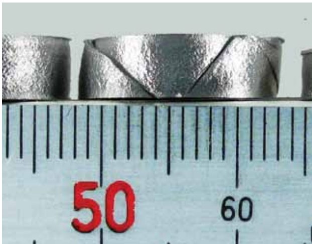
Sample deformed by dynamic plastic deformation showing pronounced shear bands.
