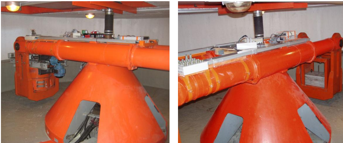
Figure 1.1 Centrifuge at DTU Byg. Left: Swing cradle for test setup. Right: Swing cradle for counter weights.
