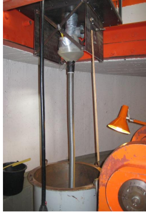
Figure 2.5 SPH setup, ready for preparation of sample.
