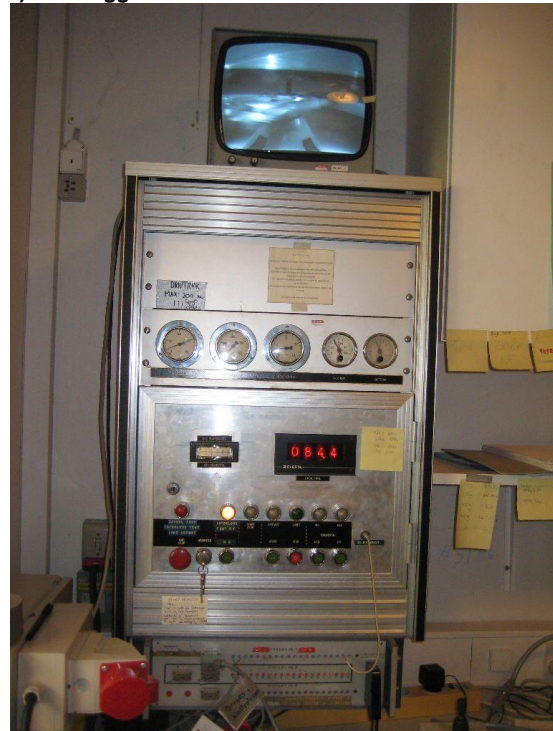
d) Main centrifuge controls.
