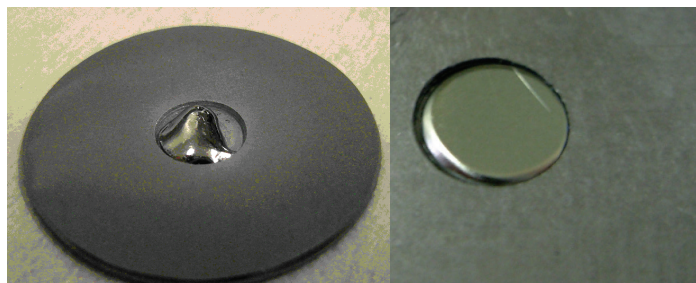
Electron beam melting of Mo to Ta target substrate
