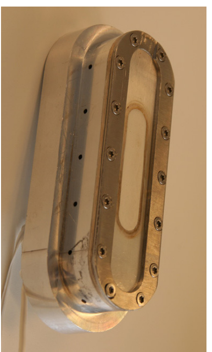
Target with electroplated Tin, - survives 200 uA
