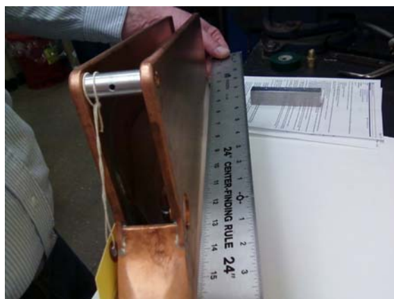
The new lower dee was installed and aligned, then removed to replace the burned fingerstock. At some point, it became bent ~2mm at the dee tip. Made of 7mm copper, it did not bend back easily. The cause is unknown.
