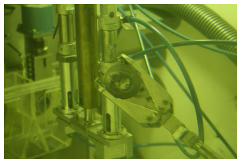
Fig 2: Broken Ga Target
