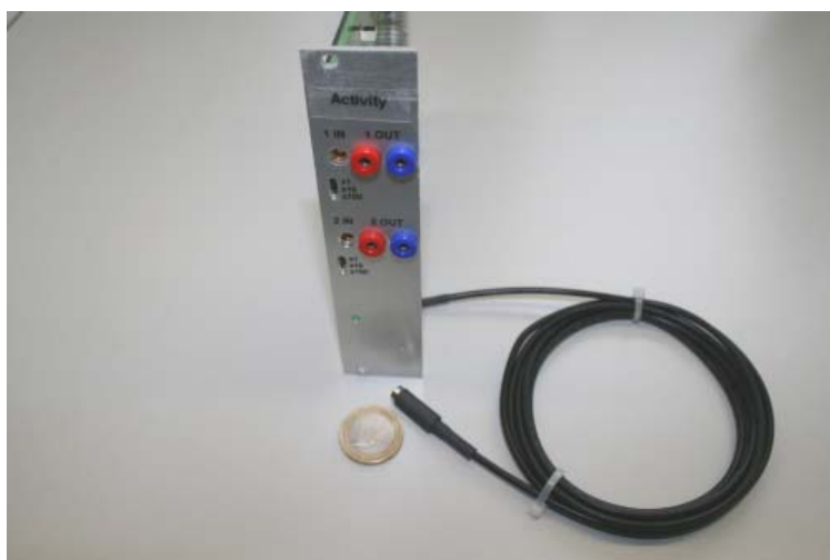
Fig. 3 Amplifier with photodiode radiation detector
