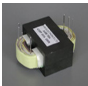
(b) Vertical winding with planar core. Search from Google
