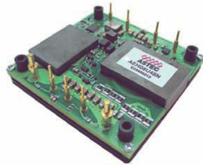
(b) 400 W Half-brick DC-DC Converter Ref. [2.32]
