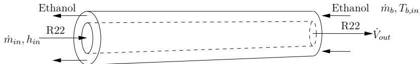
Figure 6.4: Sketch of test case evaporator
