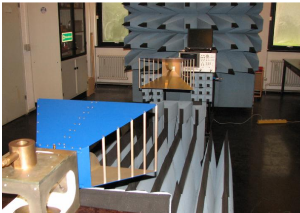
Figure 2 –The setup of the cable-free measurement technique, for two identical horn antennas.
