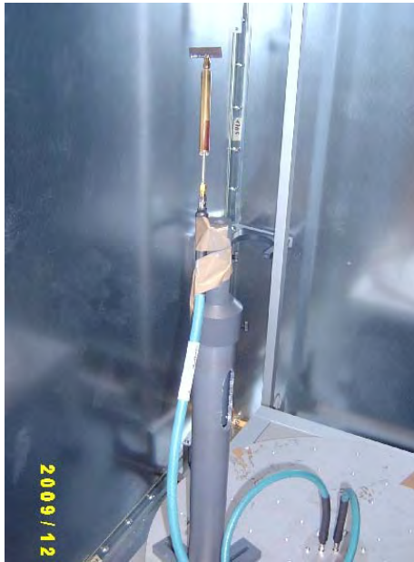
Fig. 4. The loop antenna during measurement in the reverberation chamber.
