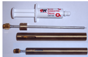
Fig. 16. Illustration of the sleeve balun and the conductive glue.
