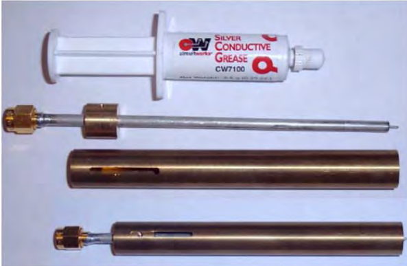
Fig. 2. Details of the tunable balun for 900 MHz.
