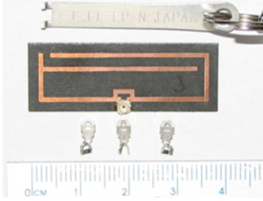
Fig. 13. The ultra small connectors and loads for the electrically small loop antenna.
