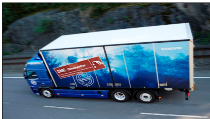
Figure 24. Volvo truck especially designed to run on Bio-DME (Volvo Bio-DME).
