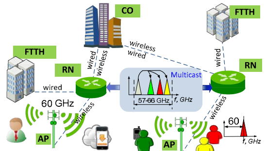
Figure 1. Network scenario for 60 GHz RoF system providing the RF tunability. CO: central office, FTTH: fiber-to-the-home, RN: remote node, AP: access point.
