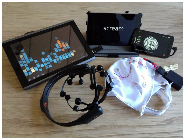
Figure 3: SBS2 mobile neuroimaging apps for neurofeedback training, presentation of experimental stimuli, and real-time 3D source reconstruction, running on Android mobile devices via a wireless connection to an Emotiv or Easycap EEG setup.
