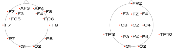
Figure 5: Electrode locations for two mobile 16 channel EEG setups; the Emotiv neuroheadset using saline sensors positioned laterally (left), versus a standard gel-based Easycap EEG montage including central and midline positions (right).
