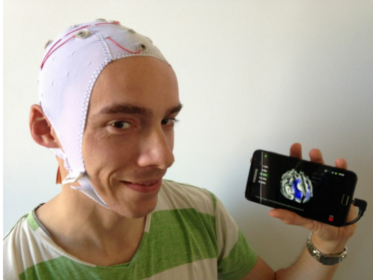
Figure 1: SBS2 mobile EEG recording with real-time 3D source reconstruction, on an Android smartphone connected wirelessly to an EasyCap 16 electrode setup based on Emotiv hardware.
