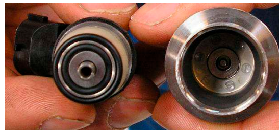
Figure 3 - Photo of disassembled injector showing O-rings
