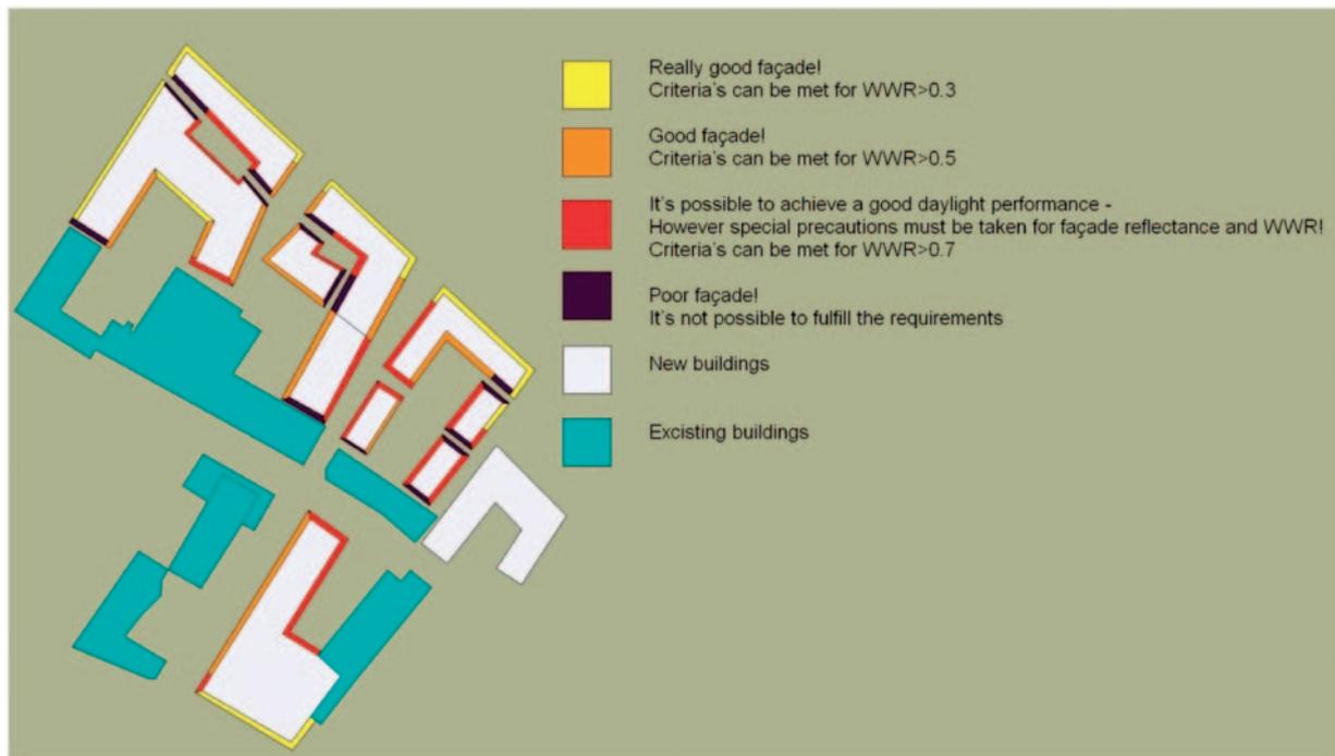
**Fig. 8.** An application example of the EvUrbanplan tool, for planning of a new urban area.
