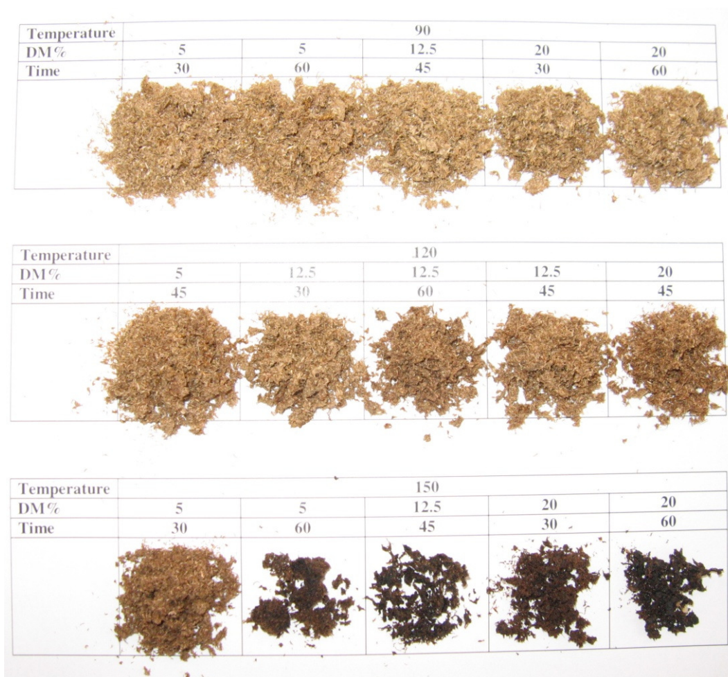
Figure 3.4 Appearance of barley straw after [EMIM]Ac pretreatment under different temperature, substrate concentration and time. Substrates were regenerated by water and then freeze dried. Values of pretreatment temperature, substrate concentration (dry matter, DM%) and time are shown in the figure.
