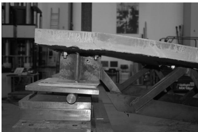
Fig. 23. Excessive deformations at support due to slip in interlocking connection between truss and anchor point.
