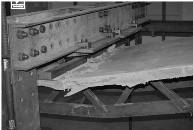
Fig. 22. A combination of compression and flexural failure during ULS testing of specimen MP4.
