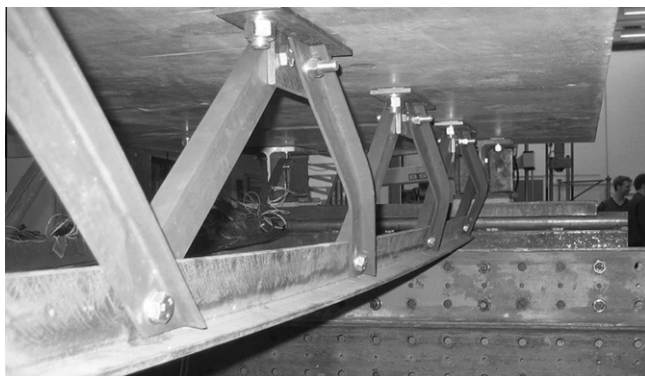
Fig. 19. Buckling of compression diagonals in specimen MP1.
