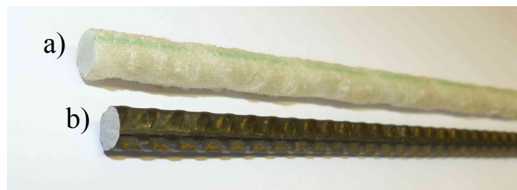
Figure 2-12 Rebars tested in this study, a) GFRP and b) standard steel.
