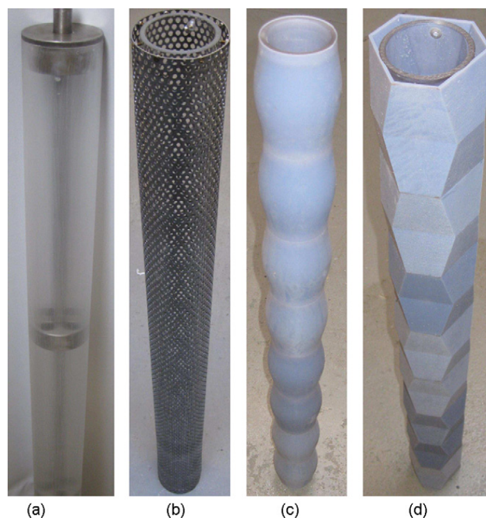
Fig. 1. Tested models. (a) Circular cylinder. (b) Shrouded cylinder. (c) Wavy cylinder. (d) Facetted cylinder.
