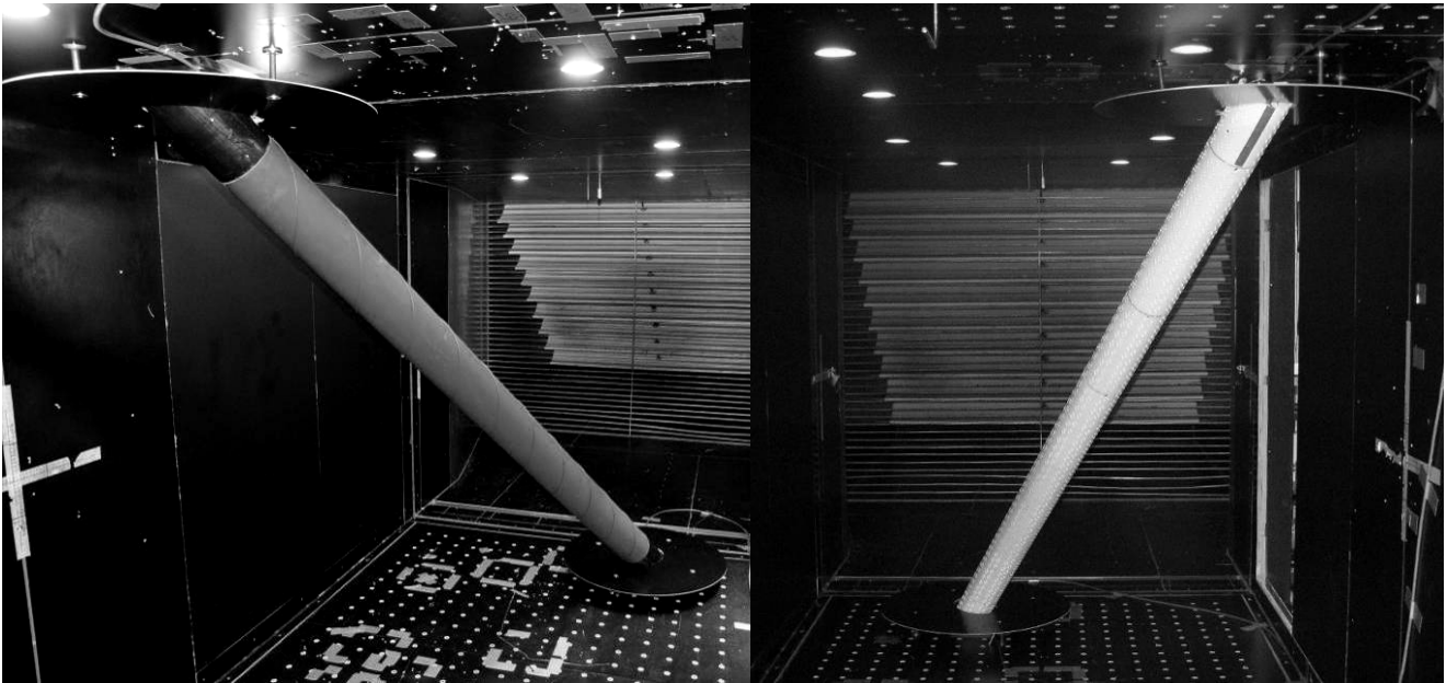
Figure 2. Yawed inclined static test setups: helically-filleted cable (left), pattern-indented cable (right).
