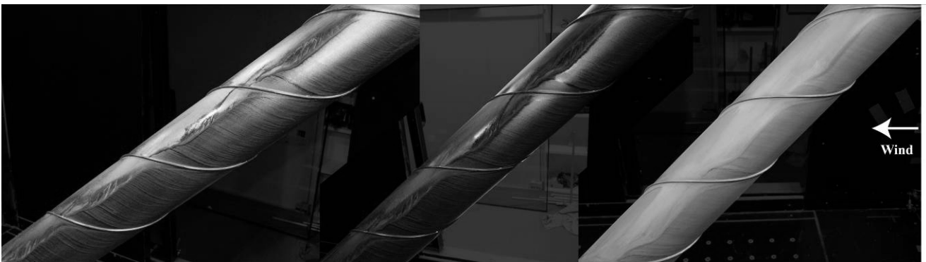
Figure 8. Oil visualization of the separation line along the left side (seen from upwind) of the helically filleted cable.
