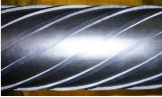
(a) Photo of test model with 12 protrusions of 5 \times 7.5 mm at \gamma = 27^\circ pitch angle. Reproduced from Yagi et al. (2010) .
