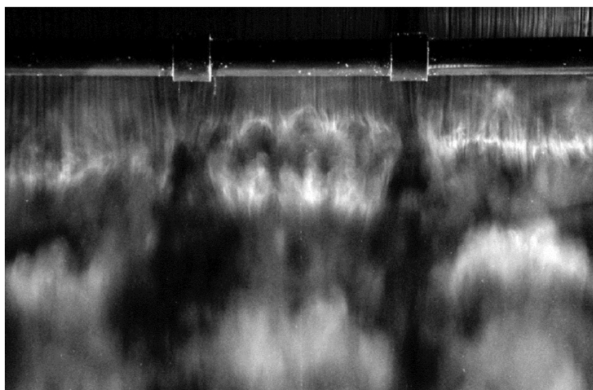
Figure 37: Near-wake flow visualization of cylinder with collars with optimal configuration. Reproduced from Nakamura and Igarashi (2008) .
