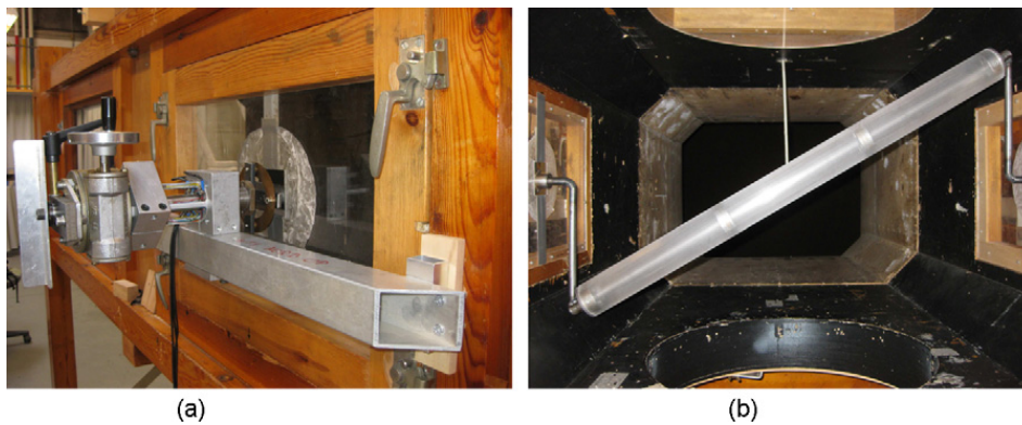
Fig. 4. Illustration of the test set-up. (a) Outside view on the testing section. (b) Section model installed in the inclined test rig.
