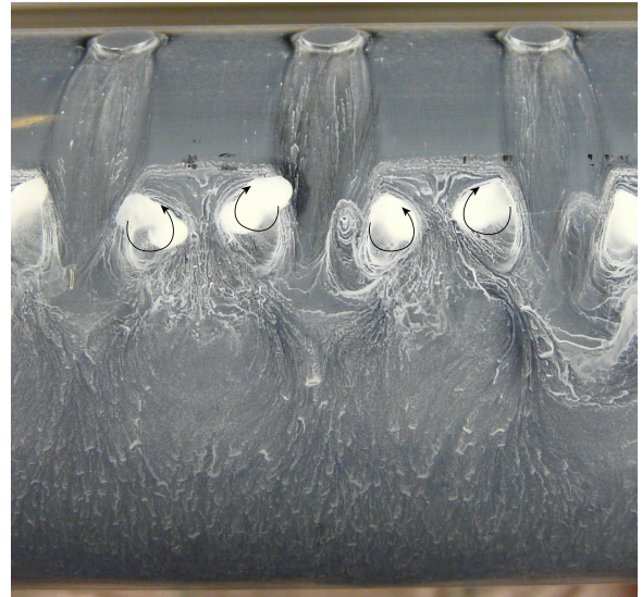
(b) Circular cylinder with CVGs at 60^\circ . Reproduced from Heine et al. (2010) .
