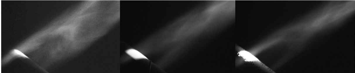
Figure 9. Near-wake smoke visualization at Re \sim 1.72 \times 10^5 : plain surface (left), helically filleted surface (middle), and pattern-indented surface (right).
