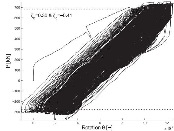
Figure 4. Load deflection result for cyclic test T3.
