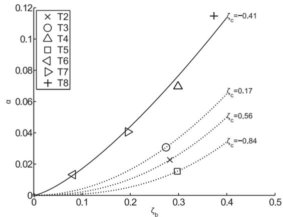
Figure 8. Rotational accumulation parameter. The value B can be found and calculated from Figure 7 in the following way.
