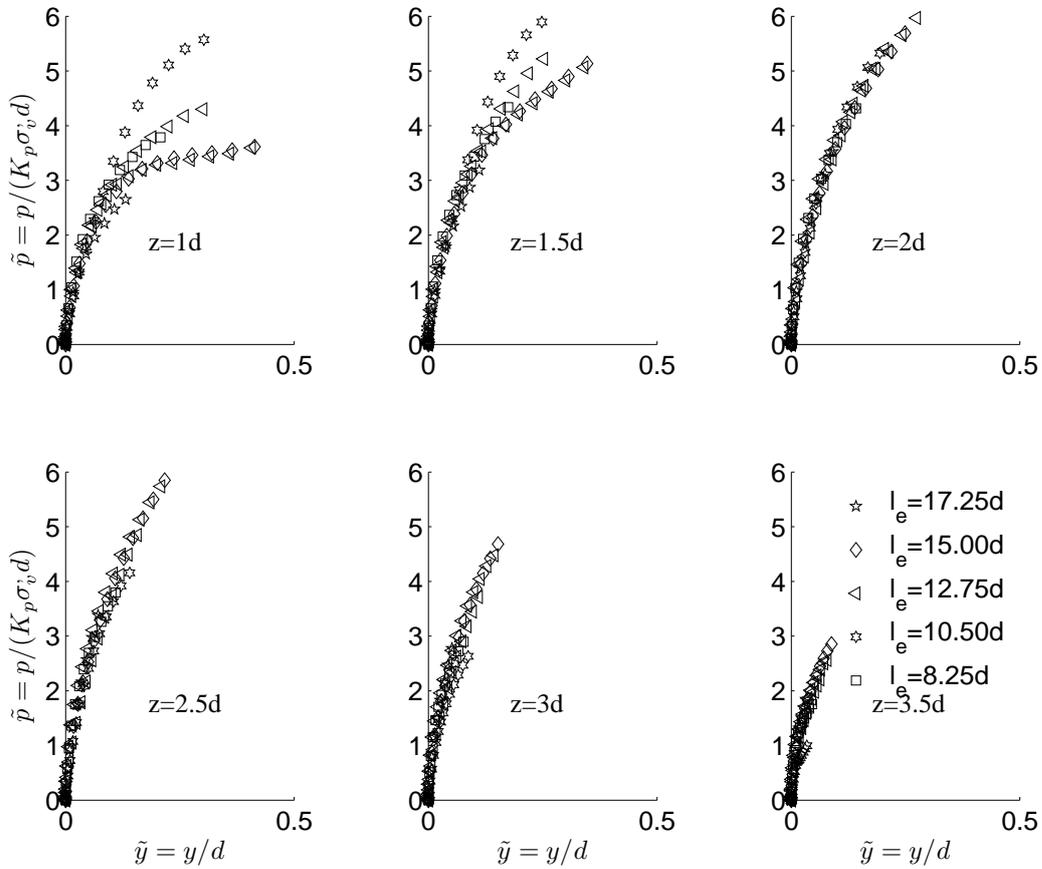
**Figure 4.5:** Monotonic test results from  $d=40\text{mm}$  pile with five different load eccentricities, Test no. 65-69
