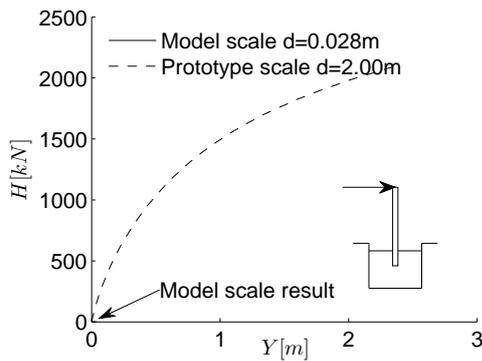
**Figure 3.3:** Abaqus calculation in model and prototype scale
