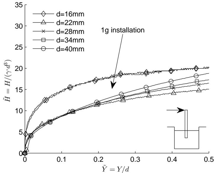
**Figure 3.13:** Grain-size effect on 1g installed piles
