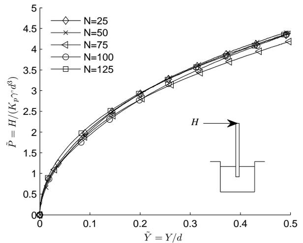
tests merge into one single characteristic curve. This indicates that the effect from stress level can as a simplification be taken into account only through the angle of friction.
