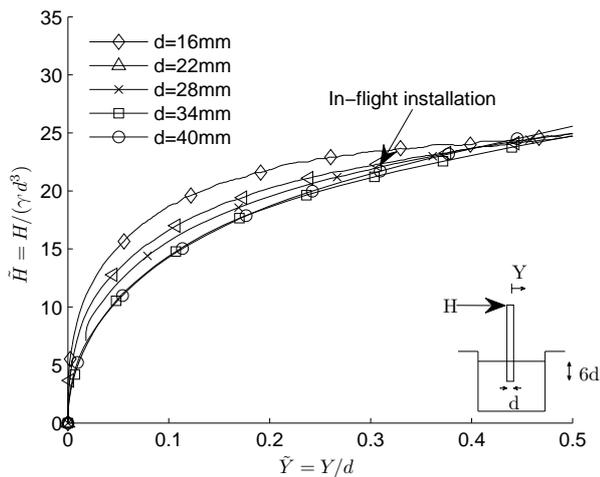
**Figure 9** Lateral loading of cylindrical piles
