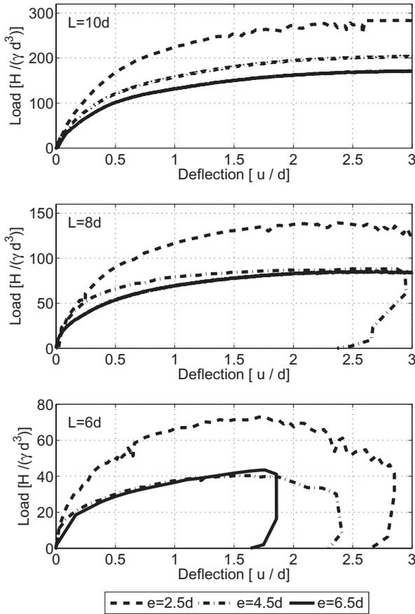
Figure 2. Normalized plot with the nine monotonic tests.
