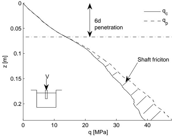
**Figure 4** Installation resistance of CPT with flat tip
