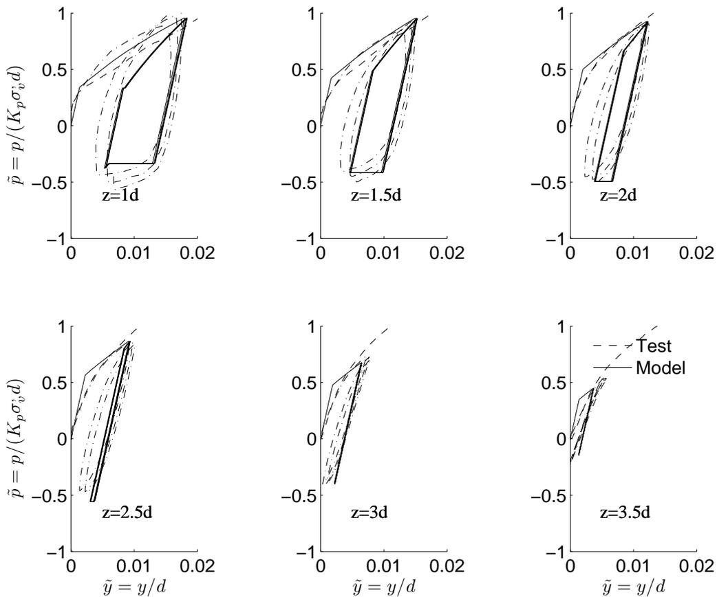
**Figure 5.6:** Comparison of the centrifuge test and Winkler model with the cyclic spring, for the local response
