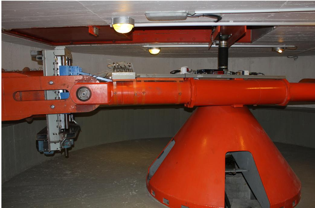
*Figure 3.5: Picture of the geotechnical centrifuge at DTU under testing*
