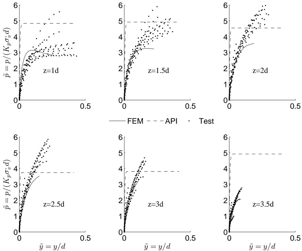
**Figure 4.6:** Monotonic test results compared with FE model and API model
