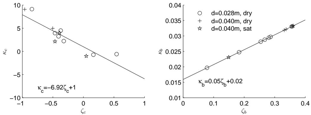
**Figure 4.15:** Non-dimensional functions to calculate the cyclic stiffness accumulation rate
