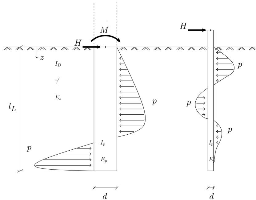
**Figure 2.4:** Monopile vs. offshore pile
