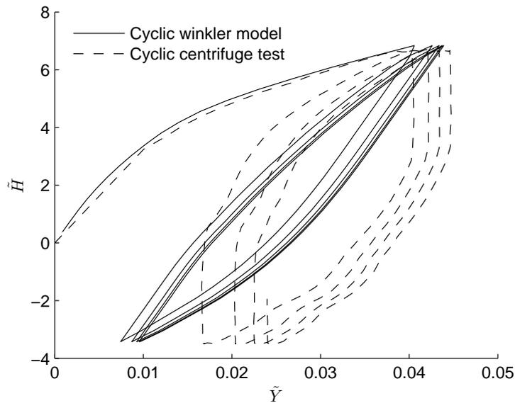
**Figure 5.5:** Comparison of the centrifuge test and Winkler model with the cyclic spring, for the overall response
