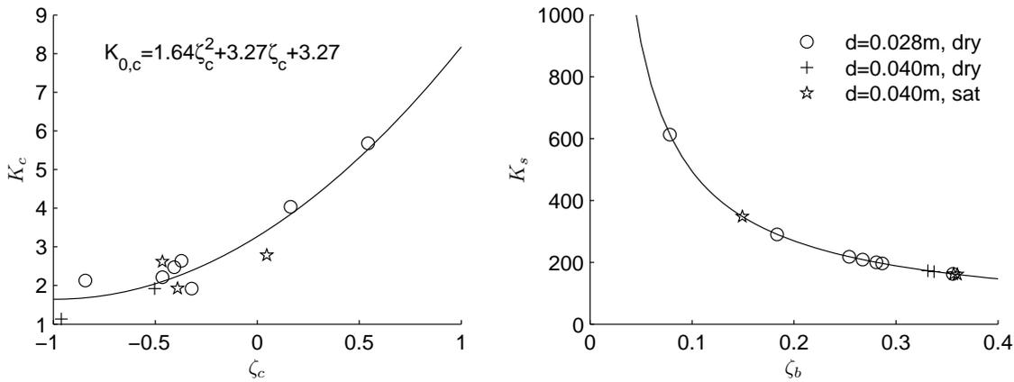
Figure 10 Cyclic dimensionless functions for initial stiffness
