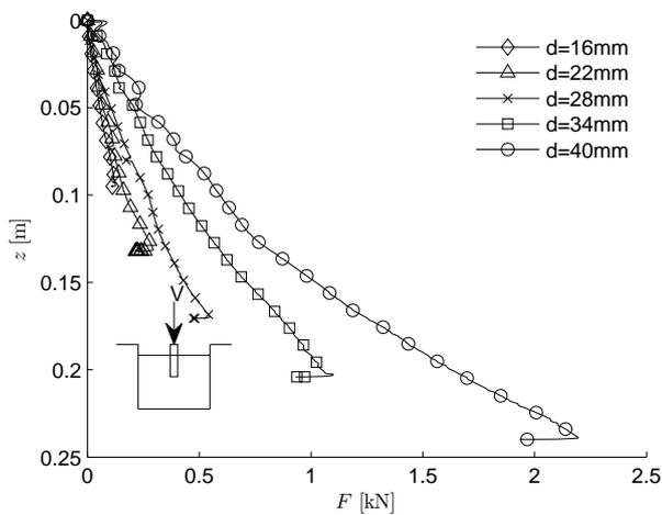
Figure 5 Installation of piles at 1g
