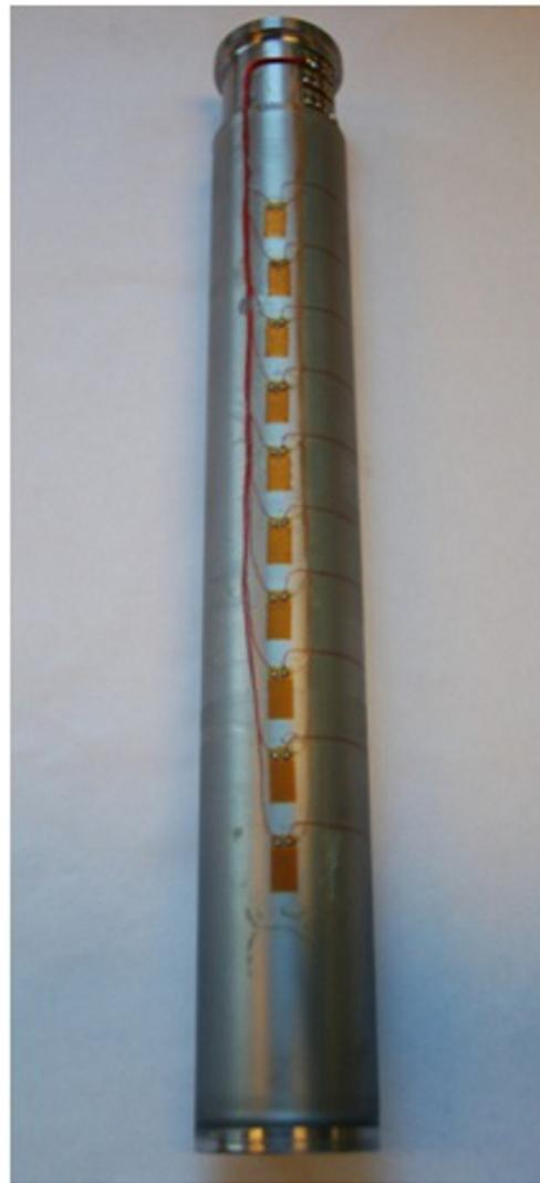
**Figure 3.10:** Photo of the model monopile mounted with ten strain-gauge half bridges
