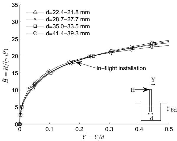
Figure 10 Lateral loading of conical monopiles
