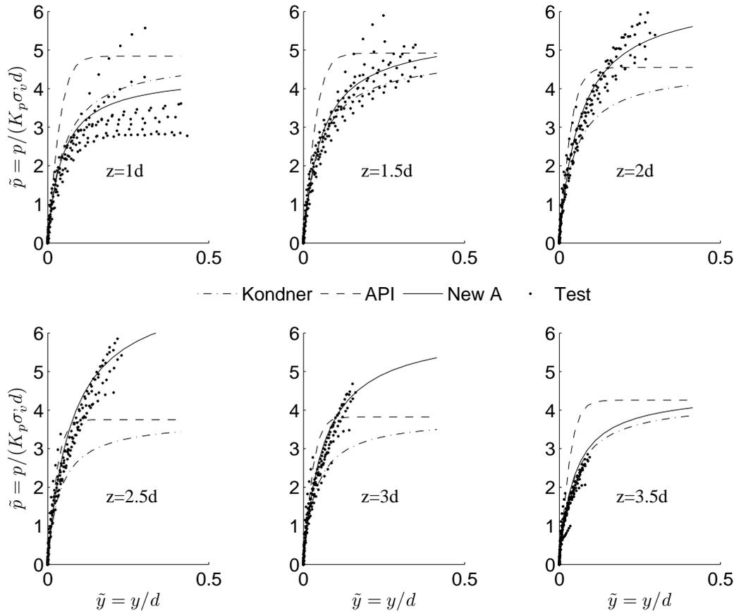
Figure 4.10: New pile soil interaction model in comparison with test data
