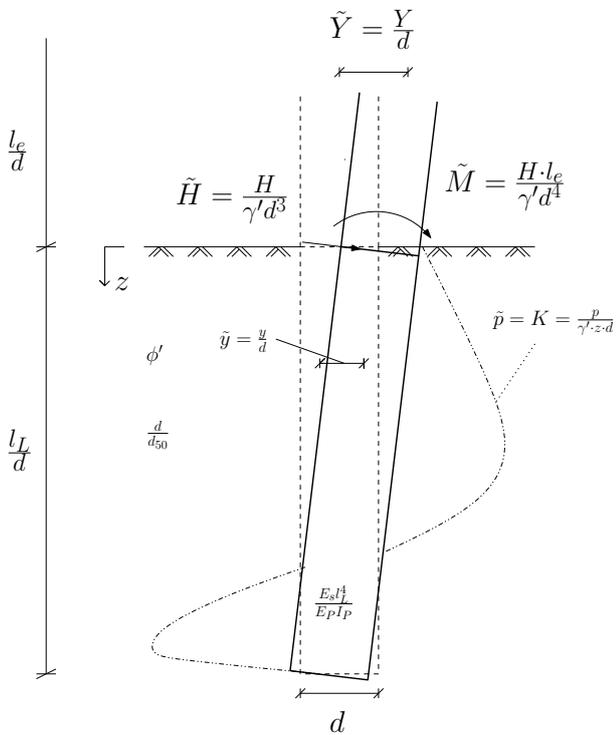
Figure 1 Sketch of non-dimensional lateral loaded pile
