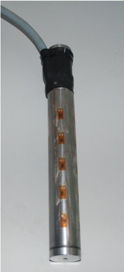
**Figure 3.9:** Photo of the model monopile mounted with five strain-gauge half bridges
