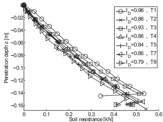
Figure 2. Monotonic test results.
