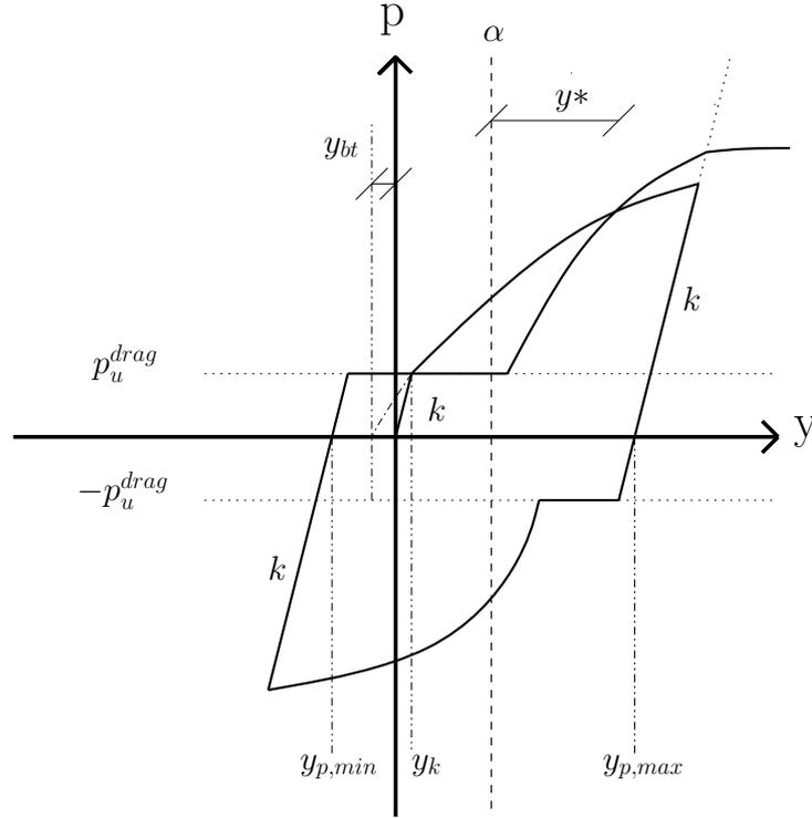
**Figure 5.2:** Schematic drawing of the spring element
