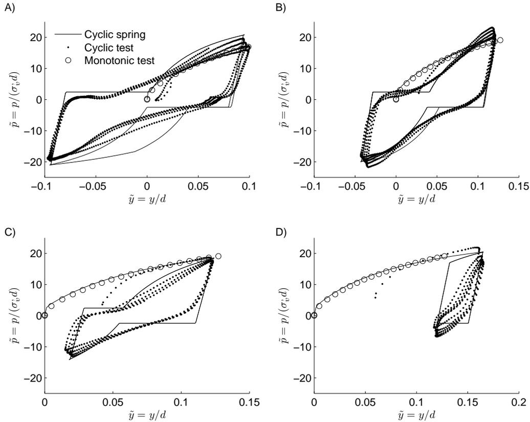
**Figure 5.4:** Demonstration of the cyclic spring,  $d=3.2m$  &  $z=2d$  &  $\phi = 42^\circ$
