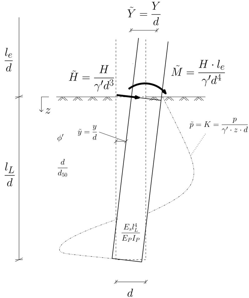
**Figure 3.2:** Sketch of pile and governing parameters
