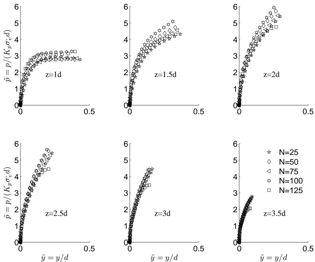
**Figure 4.3:** Monotonic test results on  $d=40\text{mm}$  pile with five different stress distributions, Test no. 26-30
