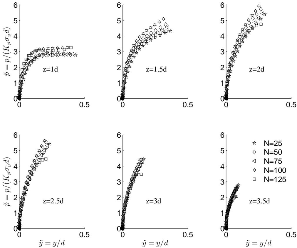
taken into account normalizing the results only using the angle of friction. These curves can then be used for any given prototype stress level, when the stress level effect is taken into account. In contrast to the API 2007 method, we use a different normalization in order to take the stress dependent maximum angle of friction into account.
