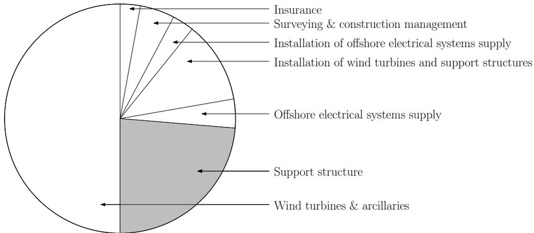
**Figure 1.2:** Schematic view of the cost of a offshore wind turbine, reproduced from: <http://www.wind-energy-the-facts.org/en/part-i-technology/chapter-5-offshore/wind-farm-design-offshore/>
