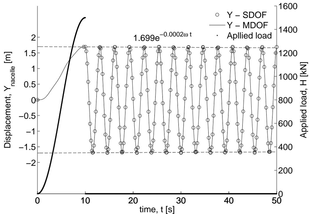
**Figure 5.9:** Free decay modelling of Horns Rev 2 wind turbine with elastic springs
