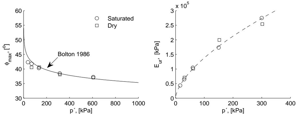
**Figure 3.11:** Results from triaxial tests on Fontainebleu sand
