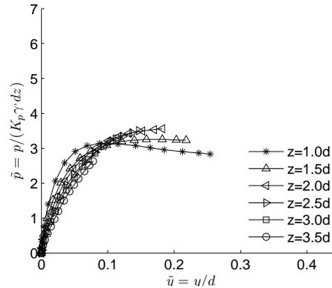
**Figure 4.8:** Pile - soil interaction curves from FE model
