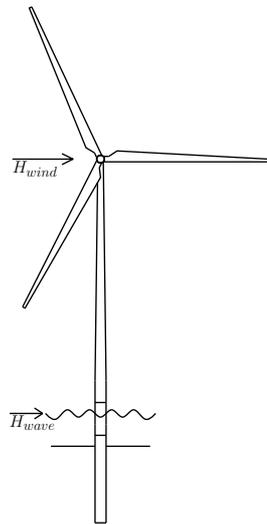
**Figure 1.3:** Force resultants on offshore wind turbine
