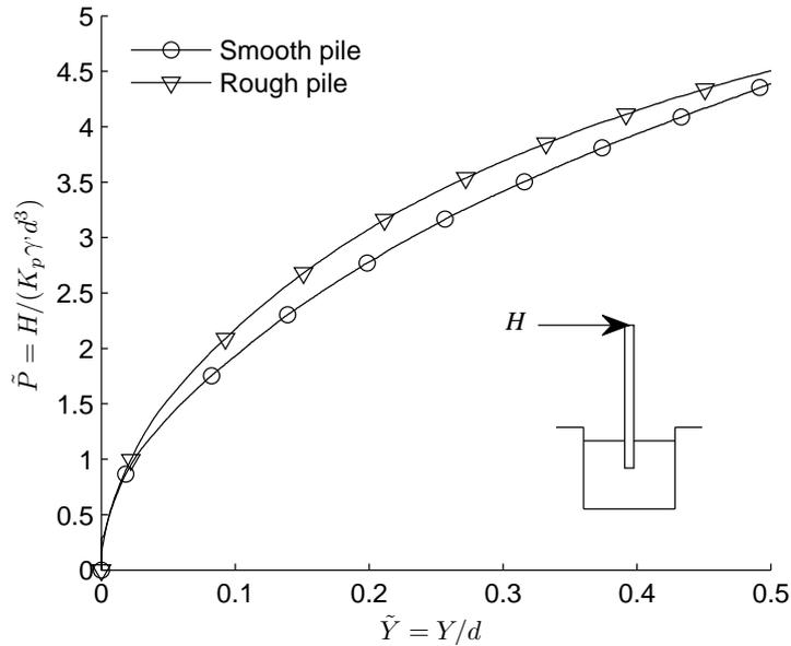
**Figure 3.20:** Effect of roughness compared to strain-gauge mounted pile
