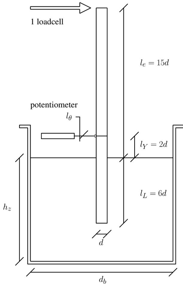
Figure 3 Sketch of the centrifuge setup
