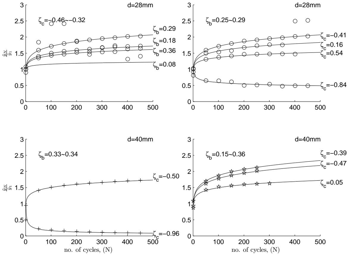
Figure 6 Accumulation of displacement from cyclic tests
