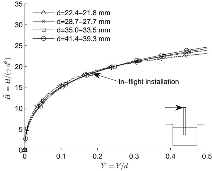
**Figure 3.16:** Effect of installation at different stress levels
