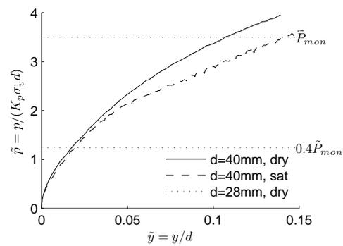
**Figure 4.2:** Pile - soil interaction monotonic response,  $z = 2d$
