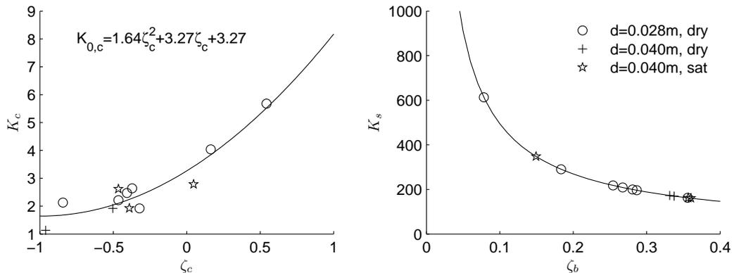
**Figure 4.16:** Non-dimensional functions to calculate the cyclic initial stiffness
