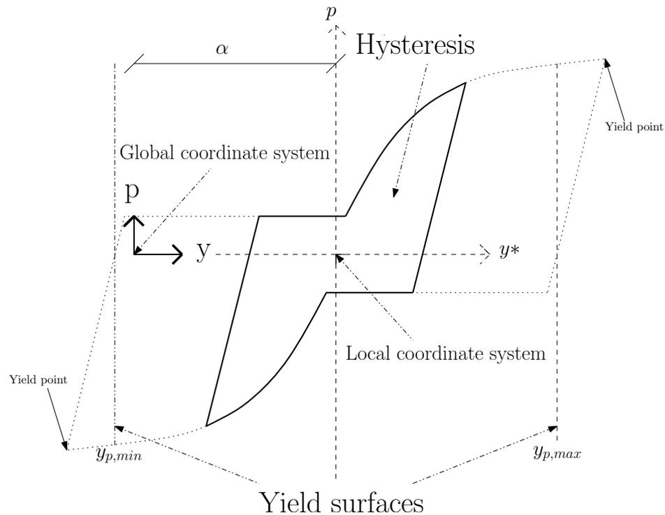
**Figure 5.3:** Schematic demonstration of the cyclic spring
