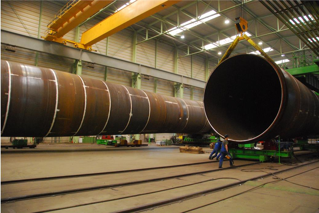
**Figure 1.5:** Picture of one of the monopiles used at Walney Wind Farm, Credit: Dong Energy
