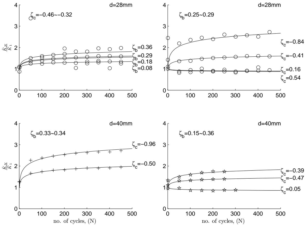
Figure 8 Change in secant stiffness from cyclic tests
