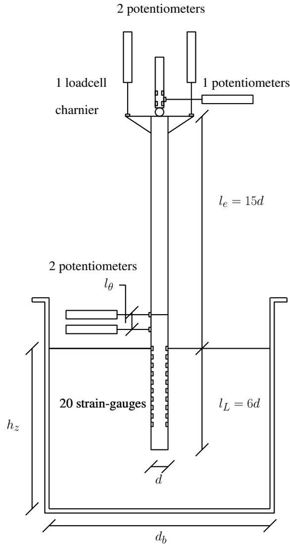
**Figure 3.8:** Sketch of centrifuge test setup
