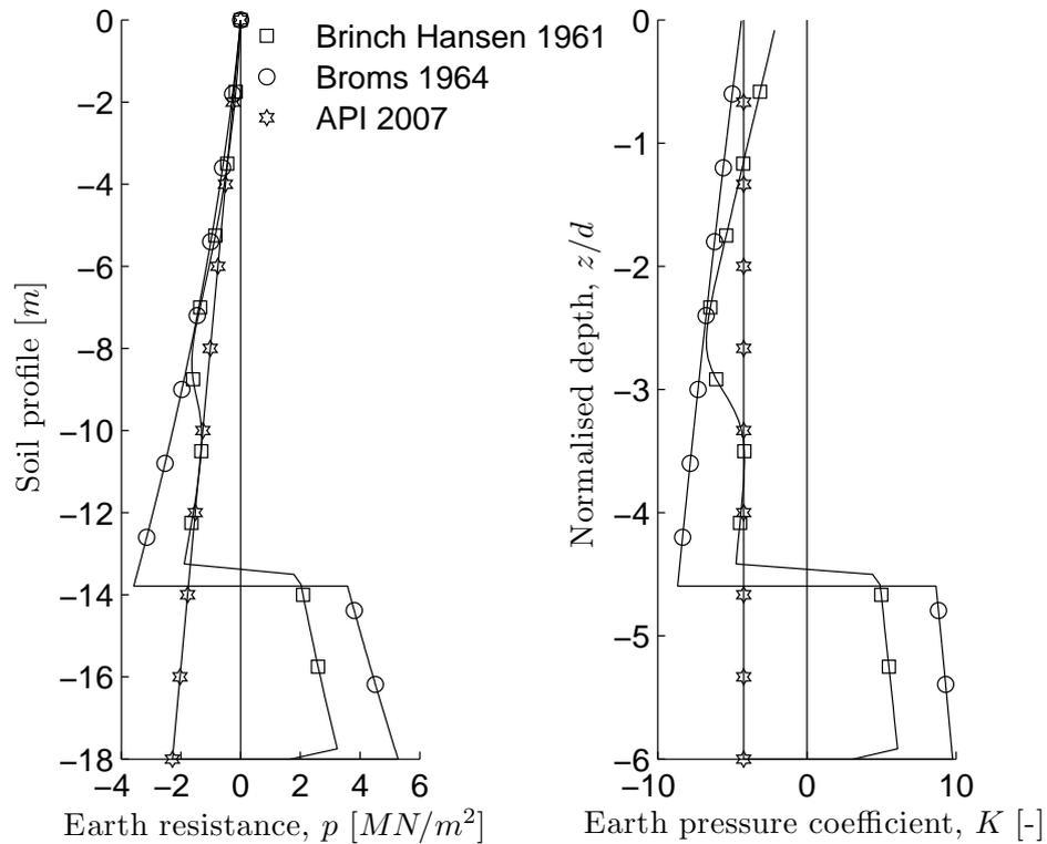
**Figure 2.1:** Comparison of soil resistance profiles at failure
