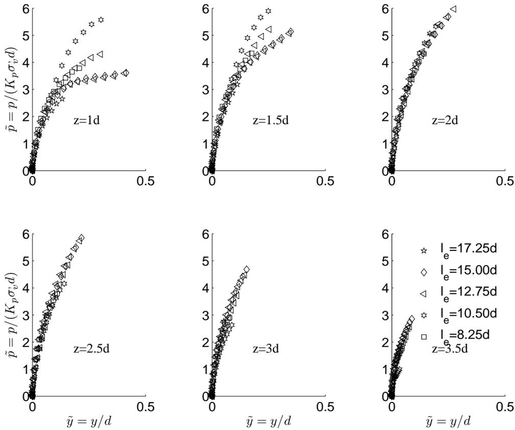
Fig. 8. Normalised general p-y curves for a pile ranging load eccentricities  $l_e = 8.25 - 17.25d$  and a diameter ranging from 1-5 m
