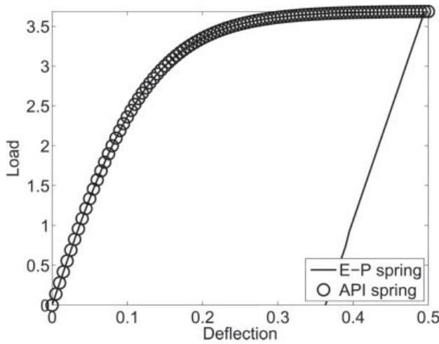
Figure 3. API curve versus the elasto-plastic curve.
