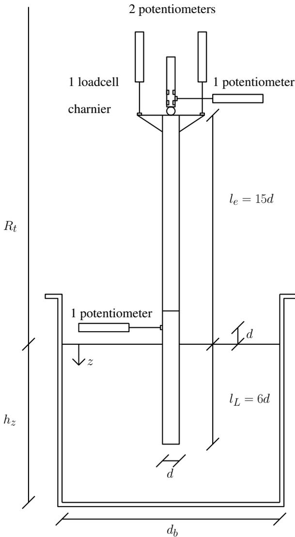
Figure 3 Sketch of the lateral load setup
