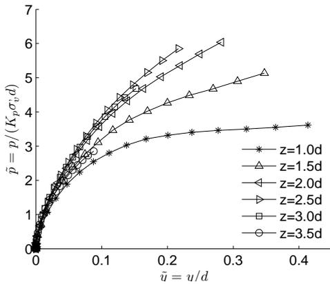
**Figure 4.7:** Generic pile - soil interaction curves from centrifuge tests
