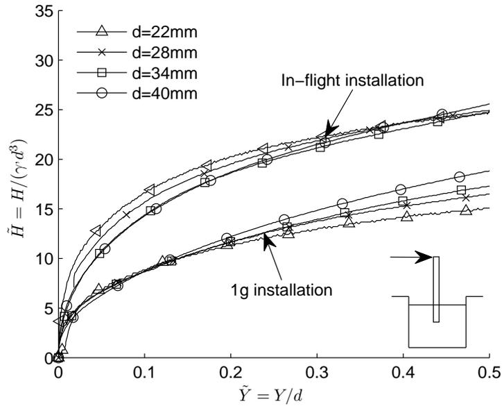
**Figure 3.14:** Effect of installation at different stress levels
