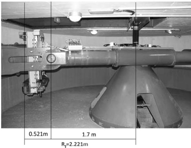
Figure 2 Photo of the beam centrifuge at DTU used for testing
