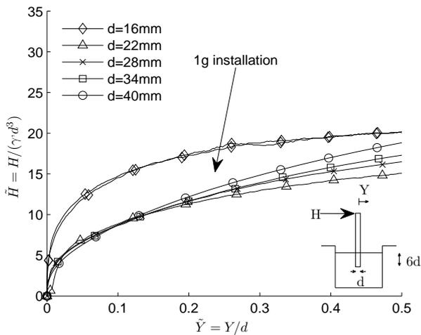
Figure 8 Lateral loading of cylindrical piles 1g installation
