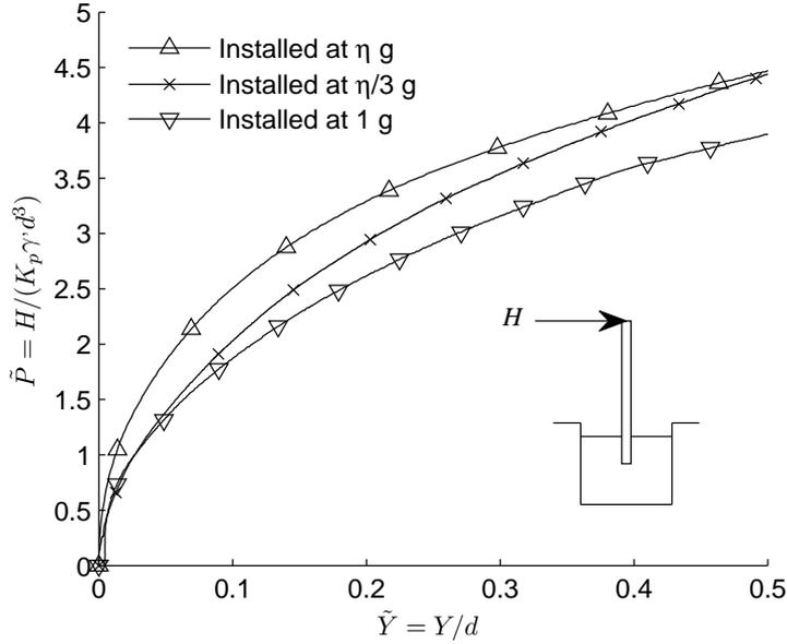
**Figure 3.21:** Effect of installation at different stress levels
