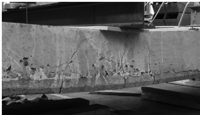
Fig. 6- Ultimate bending failure of a SL-Deck element.
