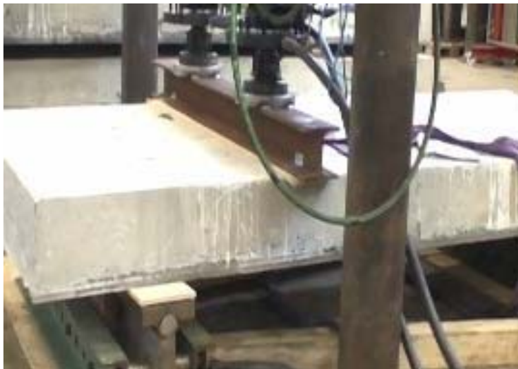
Figure 4.6: Test setup for shear test of super-light element.
