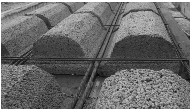
Fig. 2- Casting of SL-deck prototype test elements.
