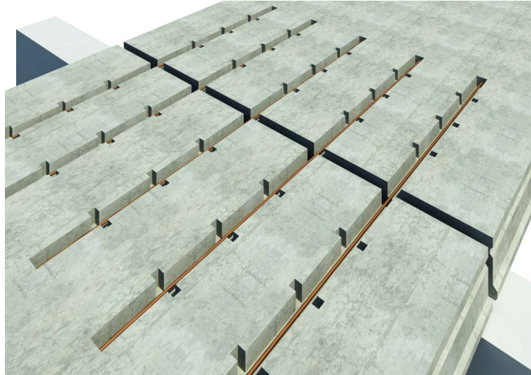
Figure 2.7: Example on how to create a restraining moment at the support in order to clamp the super-light slab.
