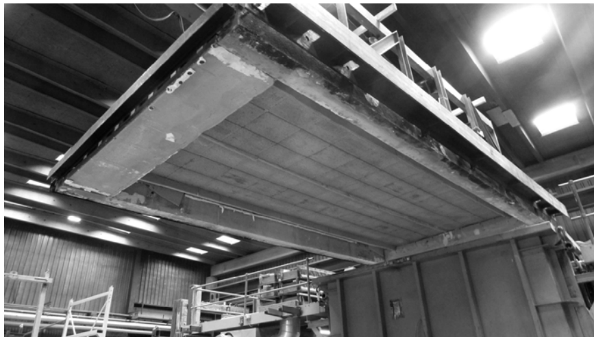
Fig. 14- Unharmed SL-Deck after 135 min standard fire exposure with 17.6 \text{ kN/m}^2 ( 367 \text{ lbf/ft}^2 ) load.
