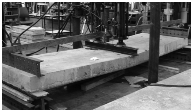
Fig. 5- Bending test rig with a SL-Deck element.
