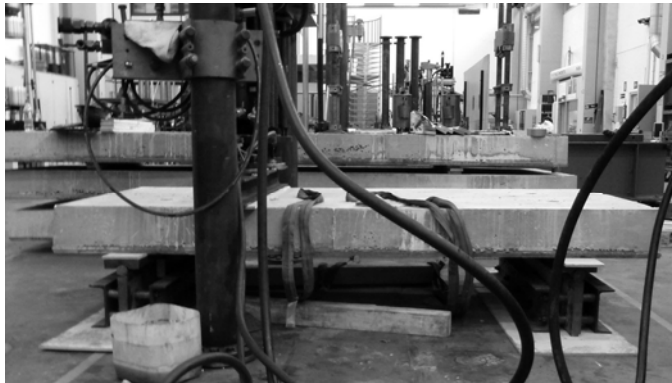
Fig. 8- Shear resistance test with a SL-Deck element.
