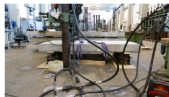
Figure 8. Shear resistance test with a SL-Deck element.
