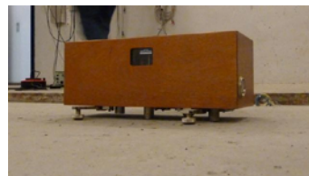
Figure 13. Impact-noise machine on a SL-Deck.
