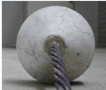
Figure 10. Conical bond test specimen with prestressing wire and cracks from fire exposure.
