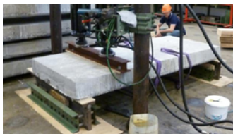
Figure 9. Pull-out test with a SL-Deck element.
