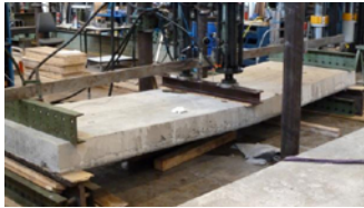
Figure 5. Bending test rig with a SL-Deck element.
