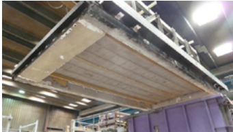
Figure 14. Unharmed SL-Deck after 135 min standard fire exposure with 17.6 kN/m 2 load.
