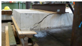
Figure 11. Pull-out test with a SL-Deck element
