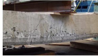
Figure 6. Ultimate bending failure of a SL-Deck element.
