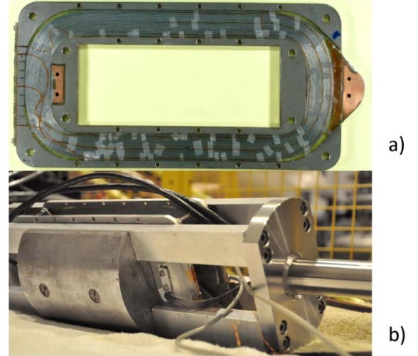
Fig. 5. a) Preview of one of the HTS coils constructed for the Superwind setup. The HTS tape is impregnated in epoxy in between SS frames. The coil terminals are made from copper blokes. They are located on the outer frame (right) and on the inner frame (left) in the end winding area of the HTS coil. The access to the 4 point measurement, the hall probes and the temperature sensors are located on the outer frame of the coil (left). Twisted pairs of wires have been soldered to the HTS tape during the winding procedure (at the beginning, end and middle of the winding). b) The HTS field winding during assembly. Two HTS coils, aluminum holders, Steel 37 pole shoe, current leads can be seen on the rotor as illustrated in Fig. 1b.
