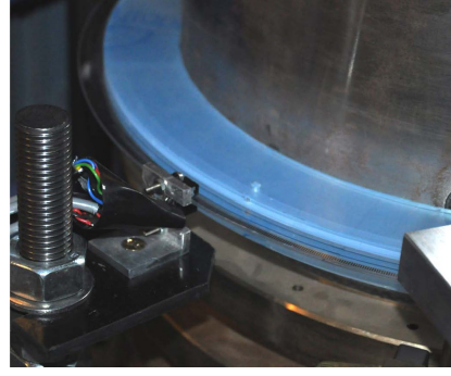
(b) Assembled encoder mounted on armature housing
