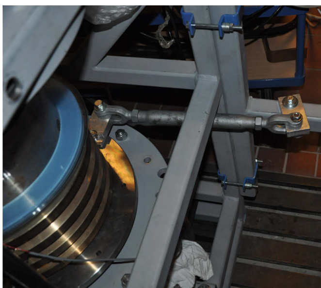
Figure 4.25: Armature winding lock assembly -
