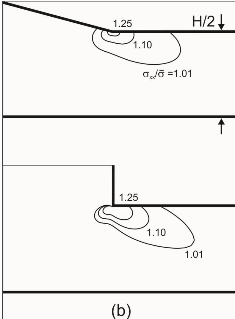
**Figure 4.17.** The stress distribution (a) as a function of the distance from the wedge tip of the tab and test material are presented with the axial stress  $\sigma_{xx}$  contours (b) for  $\theta = 15^\circ$  and  $\theta = 90^\circ$ .
