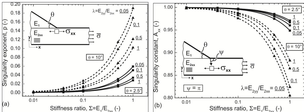
Fig 12: Stress singularity exponent ( $p$ ) and constant ( $A$ ) as a function of the stiffness ratio,  $\Sigma$  for different orthotropy parameters,  $\lambda$  in isotropy - orthotropy material combination
