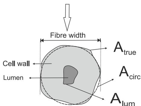
**Fig. 3** Schematic drawing of the cross-sectional fibre areas that were determined by the two different methods (Methods 1 and 2)
