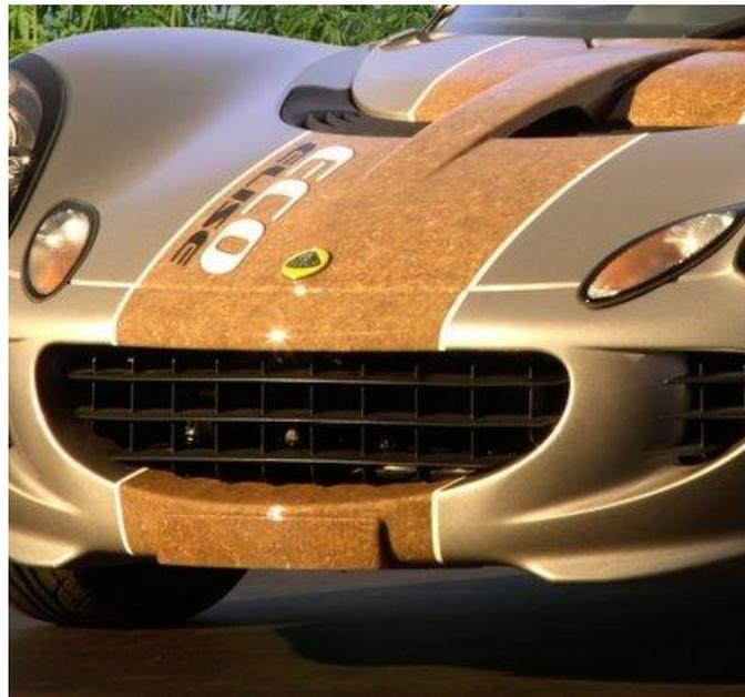
**Figure 2.6** A car body (Lotus eco) produced with plant fibre composites ([www.lotuscars.com](http://www.lotuscars.com), 2012).
