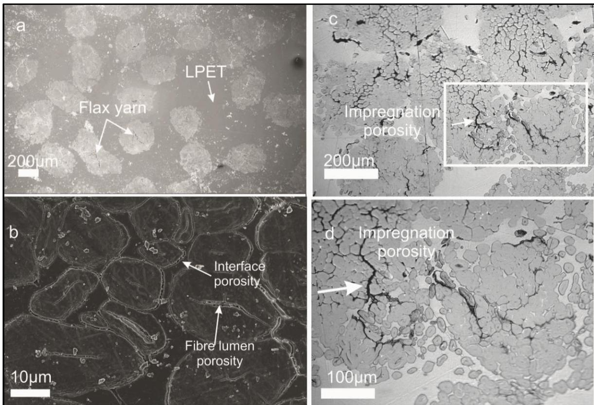
**Figure 4.4.** SEM micrographs of cross sections of flax/LPET composites: a) flax yarn distribution within the LPET matrix, b) single flax yarn with impregnation porosity, c) interfacial porosity and fibre lumen porosity, d) impregnation porosity at high magnification (white box).
