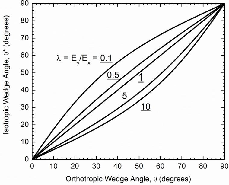
Fig 11: The rescaled isotropic wedge angles as a function of the orthotropic wedge angle,  $\theta$  for different values of the orthotropy parameter,  $\lambda$
