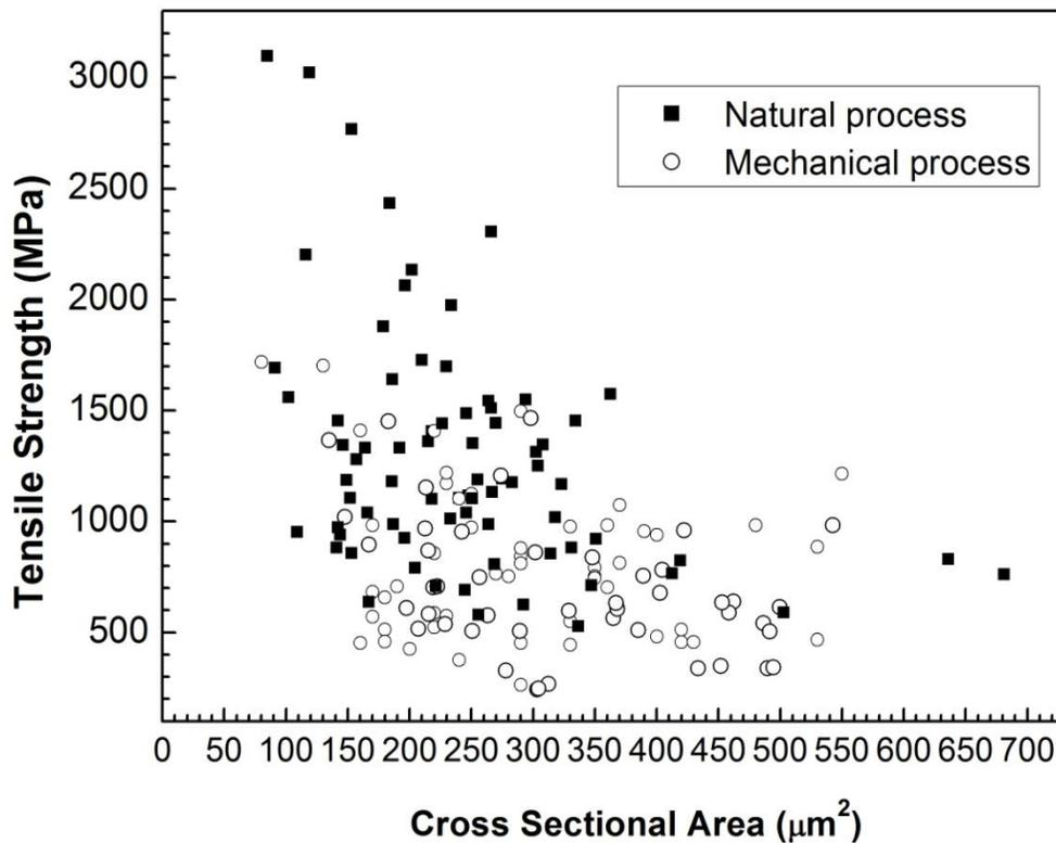
**Figure 3.6.** Tensile strength of single flax fibres as a function of cross sectional area for naturally and mechanically processed flax fibres.
