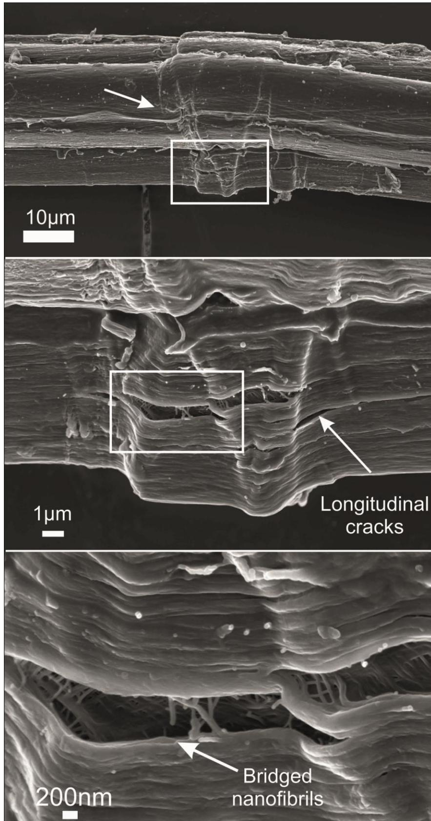
**Figure 3.2b.** SEM micrographs of surfaces of fibre bundles. The defect (kink band) zones are magnified in the white boxes and the bridged nanofibril formations are shown through the longitudinal cracks with white arrows.
