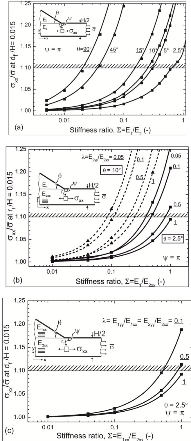
Fig 14: Stresses at  $r/H = 0.015$  corresponding to one fibre diameter for  $\theta = 2.5$  as a function of stiffness ratio,  $\Sigma$  and orthotropy parameter,  $\lambda$  for different material combinations a) isotropy-isotropy, b) isotropy-orthotropy c) orthotropy – orthotropy.
