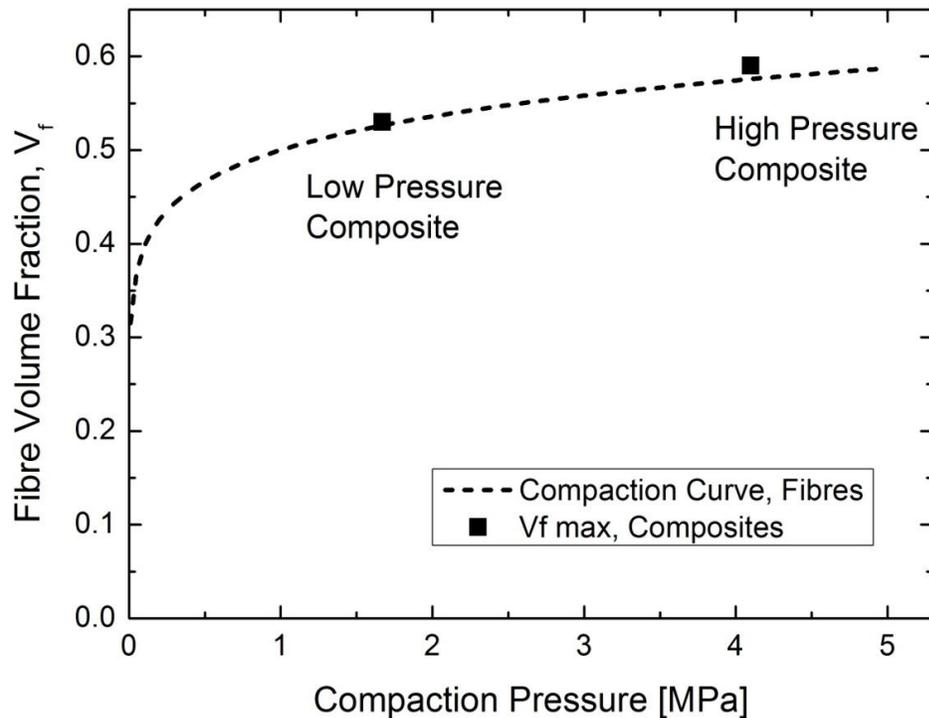
Figure 8: Compaction curve for unidirectional flax yarn assemblies together with values of  $V_{f \max}$  for the unidirectional flax/PET composites manufactured with two different consolidation pressures.
