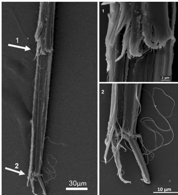
**Fig. 11** Scanning electron microscope image of a large fracture zone in a single flax fibre. Magnified views (1 and 2) are presented to highlight the longitudinal cracks along the fibre, and the formed microfibrillar units at the inner layers at both fractured ends
