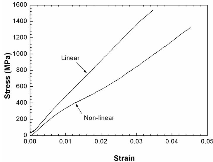
**Figure 3.** Representative stress-strain curves of single flax fibres.
