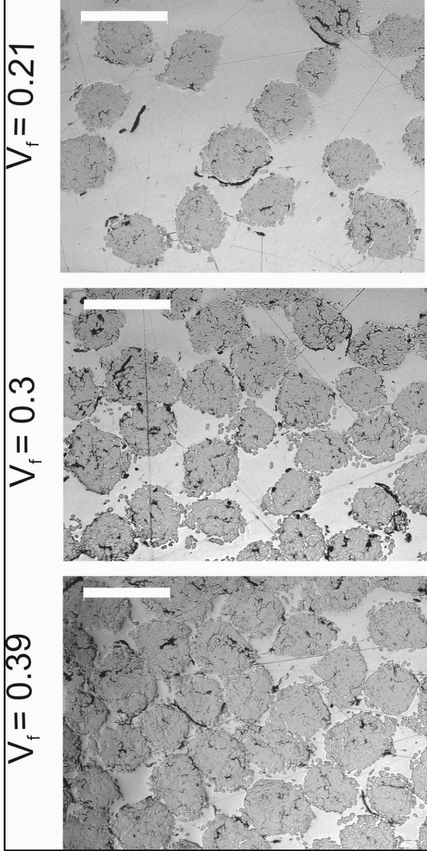
**Figure 4.3.** Cross-sectional view of unidirectional flax/LPET composites with 6 different fibre volume fractions ( $V_f = 0.21 - 0.55$ ). The flax fibres, in the form of yarns, the LPET matrix and porosities can be identified. The scale bar is 500  $\mu\text{m}$ .
