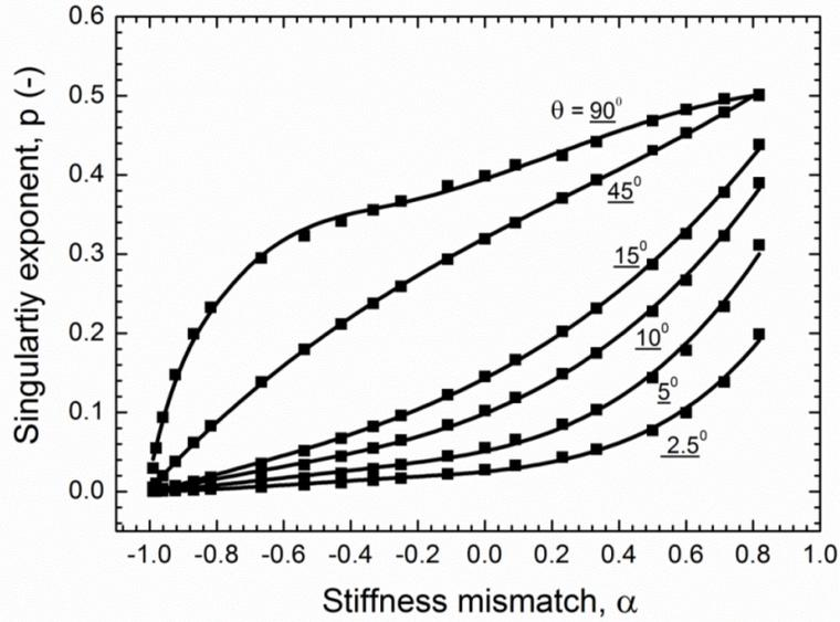
Fig 7: Singularity exponent (a) and constant (b) as a function of stiffness mismatch for different wedge angles
