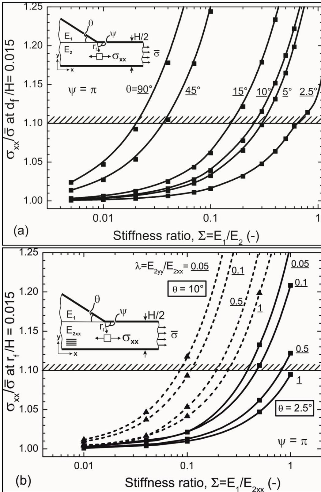
**Figure 4.19.** Stresses at  $r/H = 0.015$  corresponding to one fibre diameter as a function of stiffness ratio,  $\Sigma$  for different wedge angles in isotropic (a) and orthotropic materials (b).
