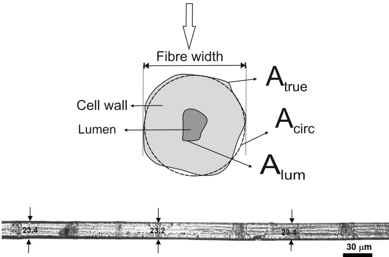
**Figure 3.3.** A schematic view of cross sectional area measurements based on the actual cross section (top) and the average width of a single flax fibre and their distribution along the fibre to calculate the fibre cross section by the circular assumption method (down).
