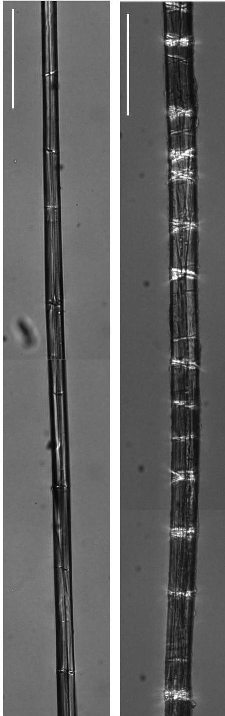
**Figure 2:** Representative images of the two types of flax fibres: Stem (left) and Noils (right) fibres. The defects can be seen as bright and dark lines across the fibres. The scale bars in both images are ca. 100 $\mu$ m.
