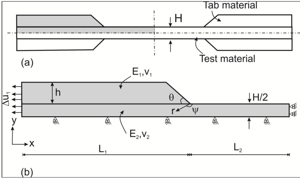
Fig 2: Schematic view of the 2D test specimen
