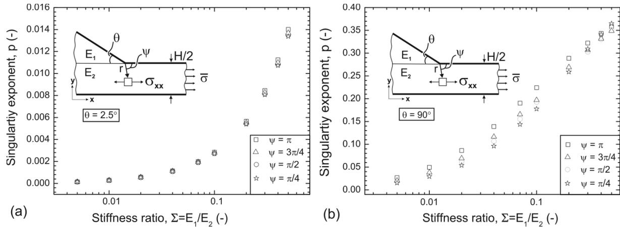
Fig. A3: The stress singularity exponents for the  $\sigma_{xx}$  stress component in  $\psi$  directions from  $\pi/4$  to  $\pi$  as a function of  $\Sigma$  for a)  $\theta = 2.5^\circ$ , b)  $\theta = 90^\circ$
