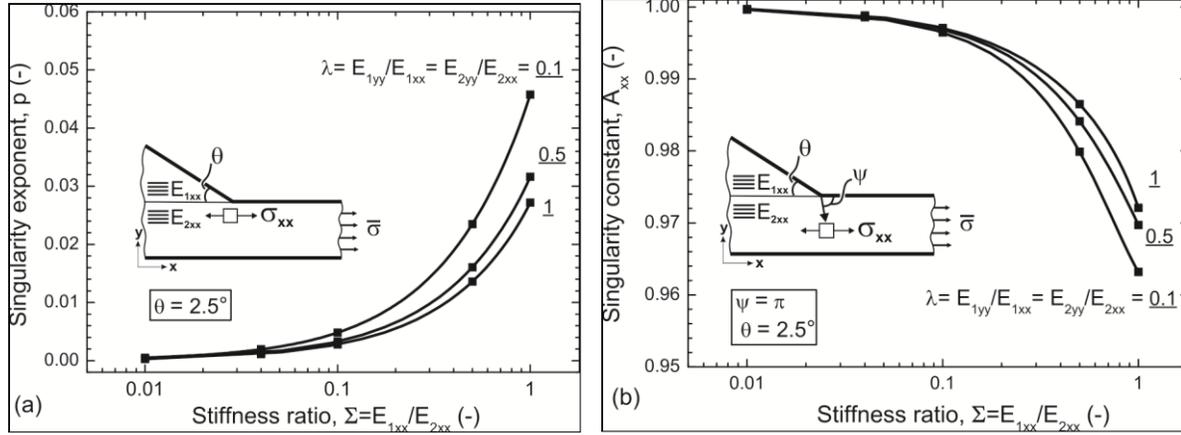
Fig 13: Stress singularity exponent ( $p$ ) and constant ( $A$ ) as a function of the stiffness ratio,  $\Sigma$  for different orthotropy parameters,  $\lambda$  in orthotropy – orthotropy material combination
