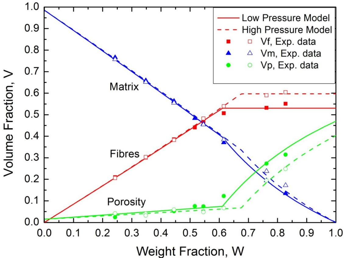
**Figure 4.5.** Model lines and experimental data points for volume fractions ( $V_p$ : porosity,  $V_f$ : fibres,  $V_m$ : matrix) of flax/LPET composites shown as a function of the fibre weight fraction. Full lines and dotted lines are used for model calculations of low and high pressure composites, respectively.
