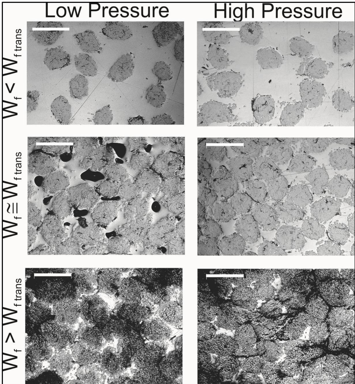
Figure 6: Optical microscope micrographs showing the microstructure of flax /LPET composites with three different levels of fibre weight fractions ( $W_f$ ), with respect to the transition fibre weight fraction ( $W_{f \text{ trans}}$ ), and manufactured with two different consolidation pressures, low and high. Values of  $W_f$  are 0.24, 0.55 and 0.76 for both the low and high pressure composites. Scale bar is 200  $\mu\text{m}$ .
