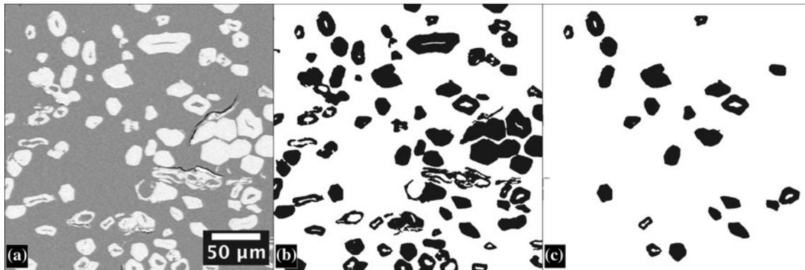
**Fig. 2** Scanning electron microscope images of flax fibre cross-sections used for the measurements of fibre area (Method 2): **a** unprocessed image, **b** binary image, **c** processed image where fibres that were not suitable for measurements were automatically removed
