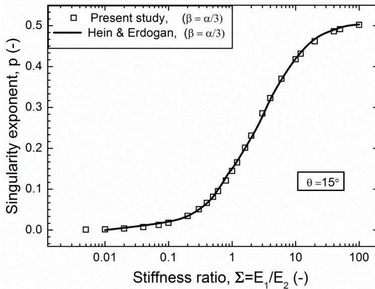
Fig. A4: A comparison of the values of the singularity exponents between the present study and a literature study [15] as a function of  $\Sigma$  from 0.01 to 100 and  $\theta = 15^\circ$  for different material thicknesses
