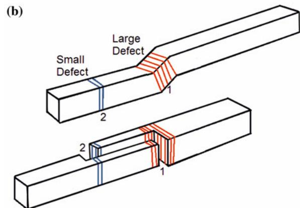
**Fig. 10** Fracture behaviour of a flax fibre showed **a** by optical microscope images of a fibre before and after fracture and **b** in a schematic view. The locations of small and large transverse defects are indicated
