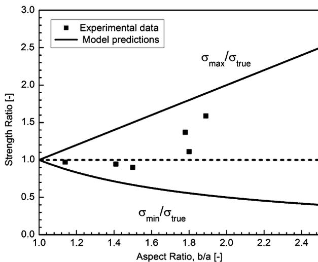
**Fig. 12** Experimental data and model predictions of the ratio between the determined strengths of fibres using the assumed circular cross-sections and the measured true cross-sections, as a function of the aspect ratio of the cross-sectional shape of the fibres
