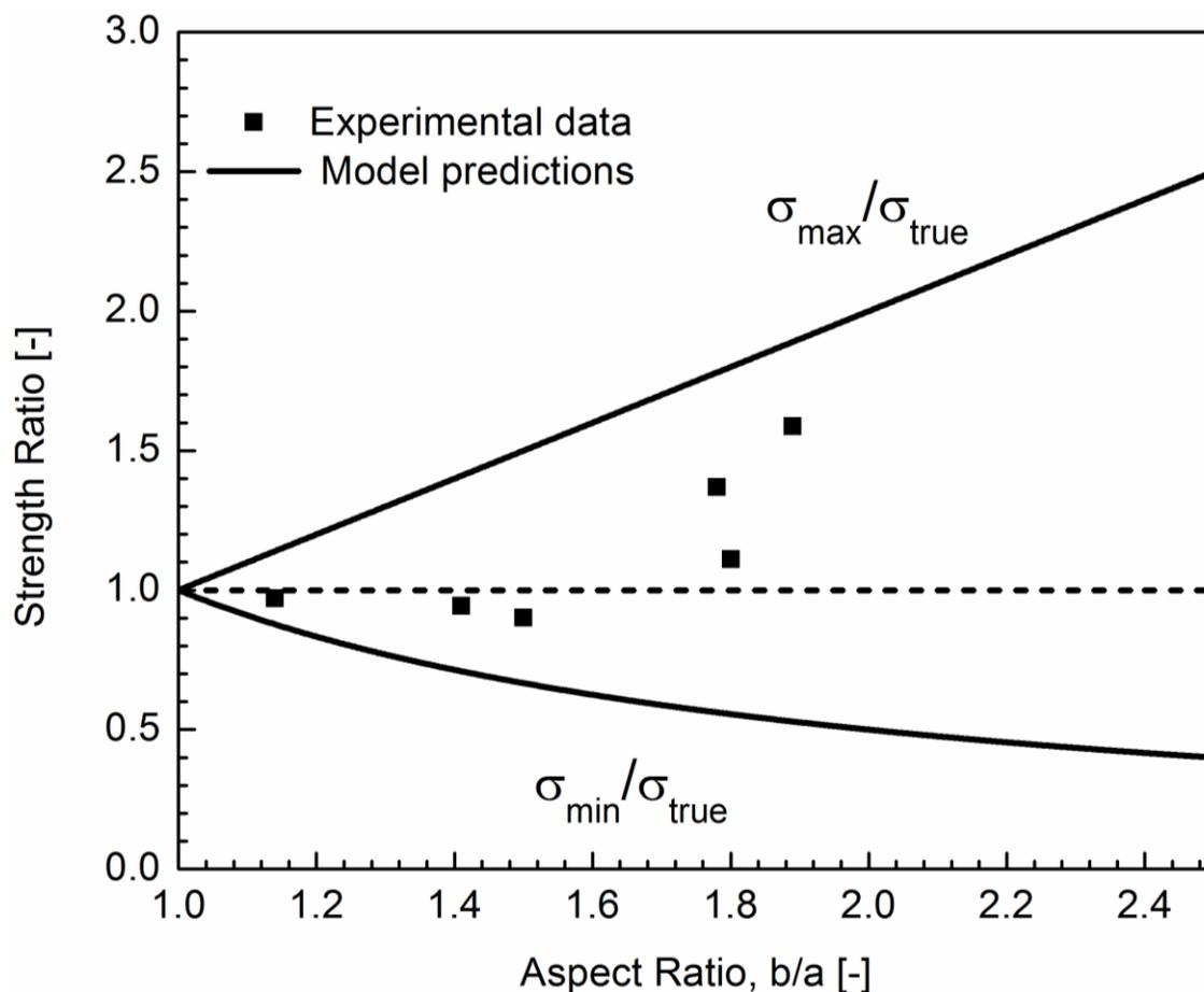
**Figure 3.9.** Experimental and model predictions of the tensile strength of fibres using the circular assumption method (maximum or minimum cross sectional area) and the true cross sectional method, as a function of the fibre cross sectional aspect ratio.
