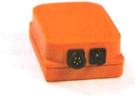
**Figure 1.1:** The sensor type used at the hands, feet, head and pelvis (lower back).
