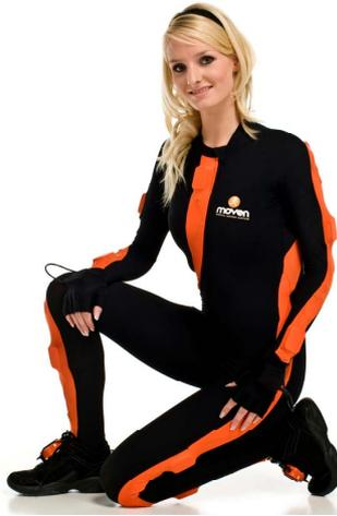
**Figure 2.5:** The Movensuit, with all sensors placed in the associated small pockets [89].
