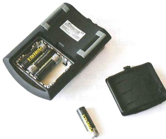
Figure 1.14: The placement of the batteries in the Xbus Masters are on the back.
