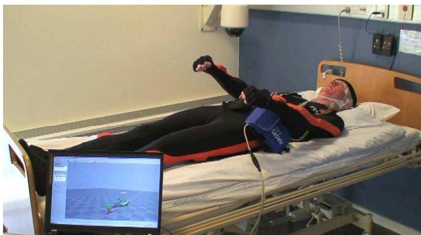
**Figure 3.1:** A control subject mounted with EEG, sEMG and the Moven system equipment, simulating a GTC seizure at the Danish Epilepsy Center in Dianalund. The Moven program is running on the laptop, showing the 3D movements of the control subject.
