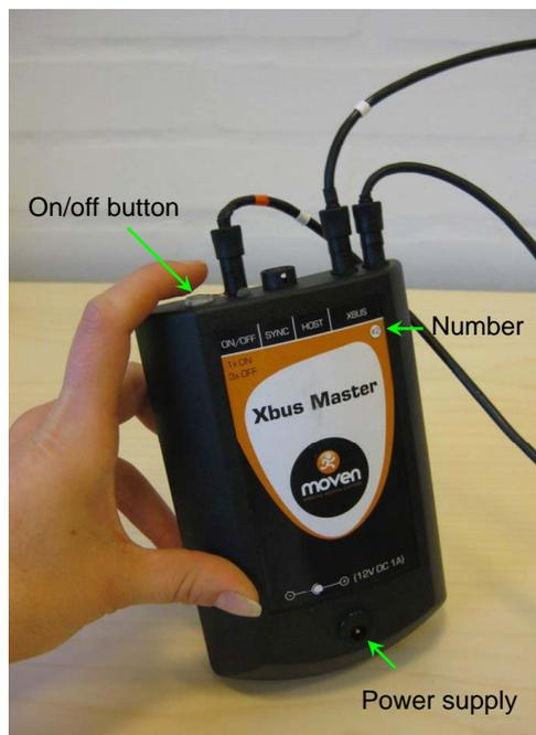
**Figure 1.7:** At the bottom it is shown where to connect the battery packages. At the top the on/off button is shown. The Xbus masters are turned on with one push and are turned off by three fast pushes. Both when the Xbus Master are turned on and when they are shut down a short beep sound will be heard.
