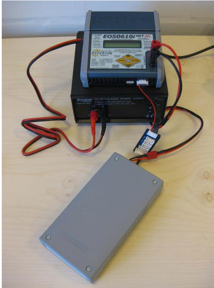
Figure 1.17: Charging of a lithium battery.
