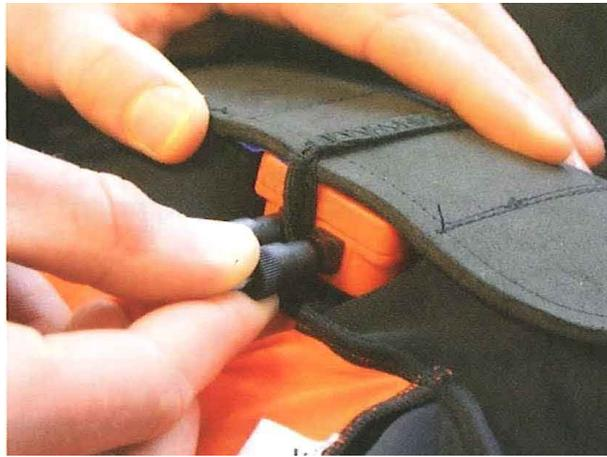
**Figure 1.6:** The placement of the sensor at the lower back (PELV). The elastic band is placed between the to sockets for the cords.
