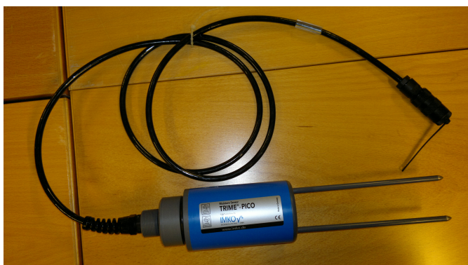
Figure D.5: Time domain reflectometry probe for measuring the moisture content of the cable surroundings.
