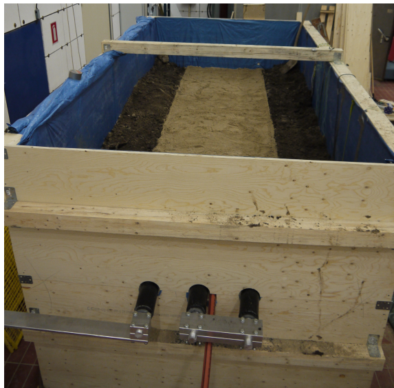
Figure D.2: Experimental setup under construction. Cables, sand and most measurement equipment is installed. A layer of soil was installed on top for completion of the setup.
