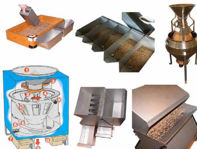
Fig. 12. Examples of mass reduction methods and devices. Top left: Spoon method (pouring); Top middle: Fractional shoveling; Top right: Boemer divider; Bottom left: Schematic of the “Vario divider”; Bottom middle and bottom right: A 10-chute and a 34-chute riffle splitter.
