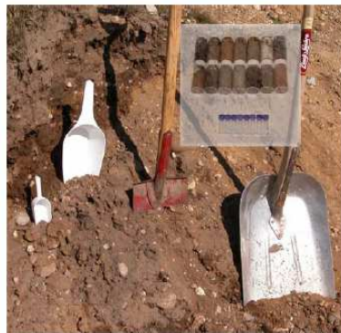
Fig. 5. What is the optimal relationship between primary sample size and the analytical sample volume (insert) and how can it come about? When sample size increases one can intuitively understand that the sample becomes more representative. But at the same time, today’s analytical volumes continue to decrease (insert) as the analytical instruments become more and more precise. For all heterogeneous materials, there is consequently an intrinsic contradiction between primary sampling representativity and the instrumental analytical volume requirements. This is the root cause of all sampling and representativity issues.
