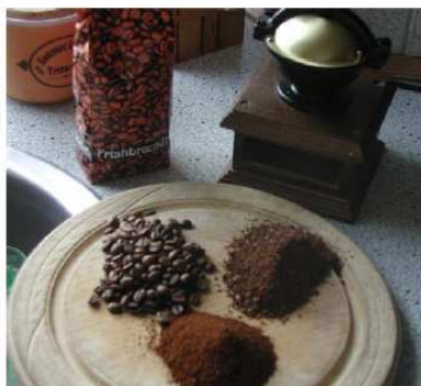
Fig. 6. Identical material composition with alternative physical grain-size states. Comminution (crushing) reduces the average grain-size, thus making it very much easier to mix and homogenize the material with a resulting significant reduction in constitutional heterogeneity. Blended coffees offer a vivid illustration.
