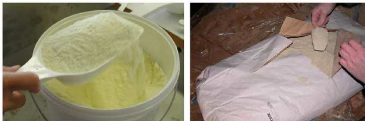
Fig. 3. Illustrative examples of grab sampling . Only the top and most easily accessible material has a chance of ending up in the final sample. This is by all accounts the most often used sampling procedure of all—and it is at the same time the worst of all sampling procedures as it blatantly ignores the Fundamental Sampling Principle FSP. TOS stresses again and again: Avoid grab sampling at all costs.
