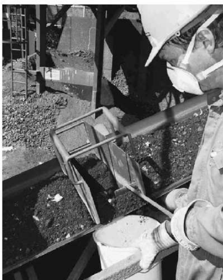
Fig. 1. “Stopped belt sampling” of bottom ash from the conveyor belt. Absolute all particulate matter in the frame is excavated, including all fines.
