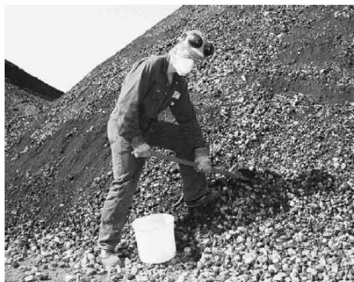
Fig. 10. Manual sampling (grab sampling) of bottom ash from a stockpile. This is the officially recommended procedure.
