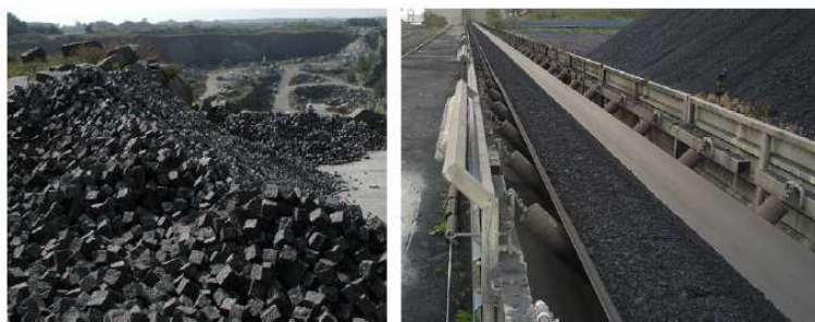
Fig. 2. Illustrations of 0-D and 3-Dim. (left) and 1-Dim. lots (right) and the scale issues in lot sampling. Note the extreme fragment size of the lot depicted in the left panel, compared to the more conventional fragment sizes relative to the dimensions of the conveyor belt in the 1-D illustration. Lots range from these macro- to meso-scale all the way down to stockpiles of fine powders.
