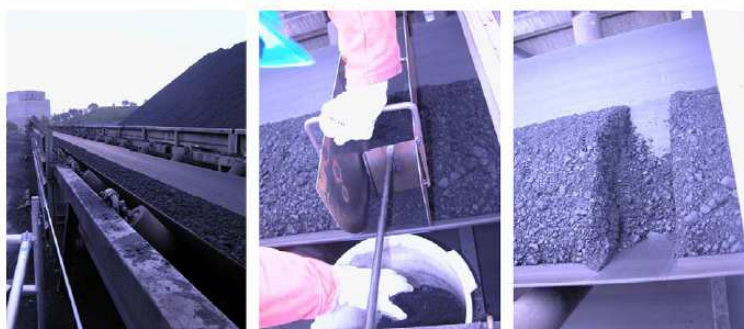
Fig. 10. Illustration of IDE. In order for IDE to be fully suppressed, the cut delineation must correspond exactly with the geometrical plan, i.e., the planar sides of the cut must be parallel and all material inside the increment must be fully extracted. In the present case, coal is sampled on a stopped conveyor belt by inserting a manual “cutter-device” and scooping out all the material (the fine particles in the groove are extracted using a brush). (The material in the rightmost panel has fallen into the “increment space” only after removal of the cutter-device.)
