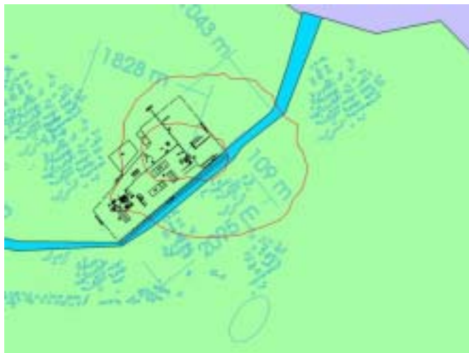
Figure 3 Discrepancy in the results of individual risk calculations: Maximum and minimum distances for the isorisk curve 10^{-5} yr -1
