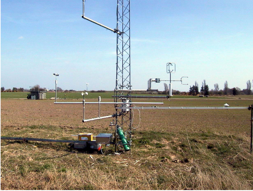
Figure 8. The RIMI experimental setup as seen from west. The cup anemometer to the far left is the Risø P2546 model. The height of the rotor is 2.2m and the boom is pointing north. The Solent three-dimensional sonic anemometer is mounted on the boom pointing in the direction 240^\circ . The middle of its measuring volume is at the height 2.3 m.
