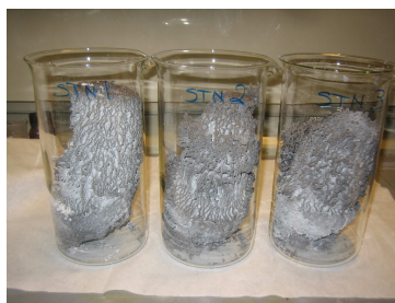
Figure 2.1: STN powder before calcination.
