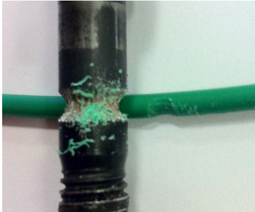
Figure 6.23: Filament Drive Axle and shredded filament wire. The teeth of the drive-axle has ground an indent in the filament.
