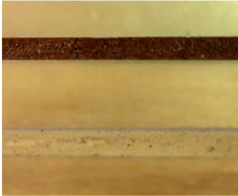
Figure 7.4: An empty and a spackled groove. Ensuring controlled and repeatable groove cross-sections
