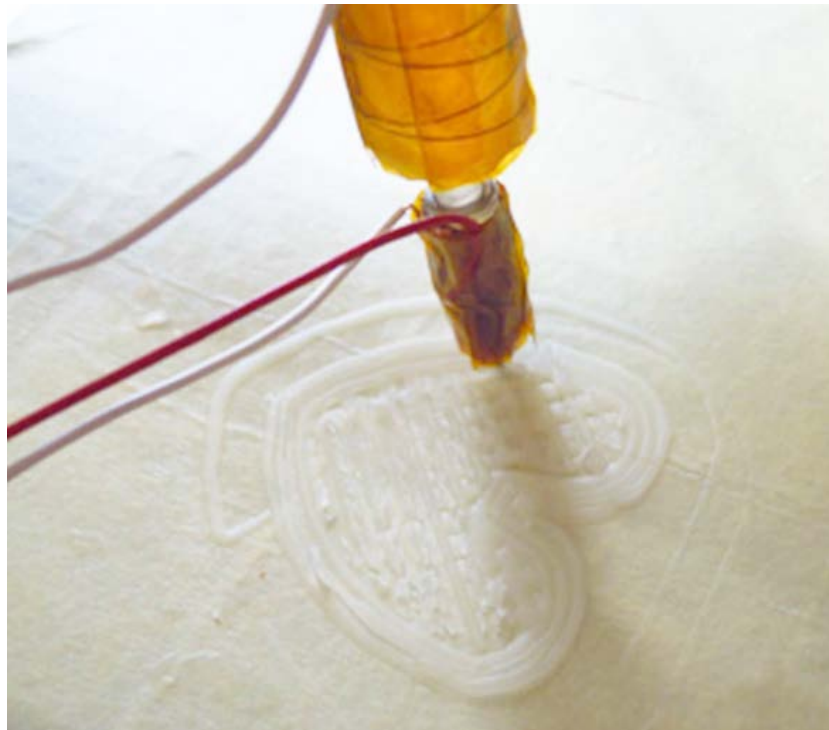
Figure 7.10: The extrusion of layered structure in paraffin wax. Thermal heating elements are employed to control the plasticity of the wax.
