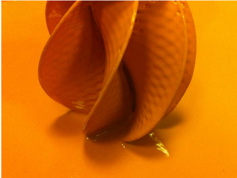
Figure 4.21: Additive Manufacturing job on an EnvisionTEC MML, DLP platform.
