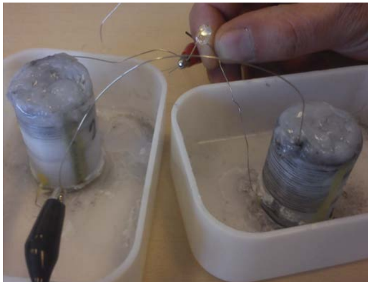
Figure 7.3: Testing battery cells: Two batteries in series powering a light emitting diode.
