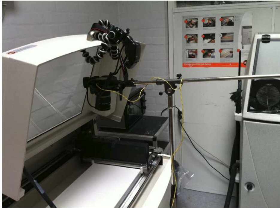
Figure 4.8: Vision system integration in a z310 plus 3DP machine. Showing a digital SLR camera on a tripod with an external flash unit mounted to the frame of the 3DP machine, and an integrated triggering wired extending from the camera.
