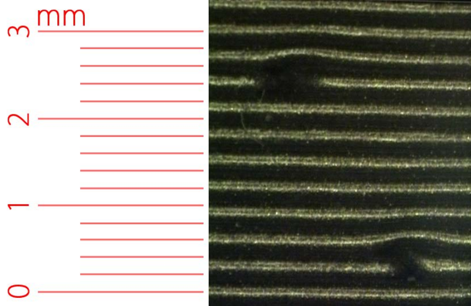
Figure 6.14: Detailed view of defects formed from layer change
