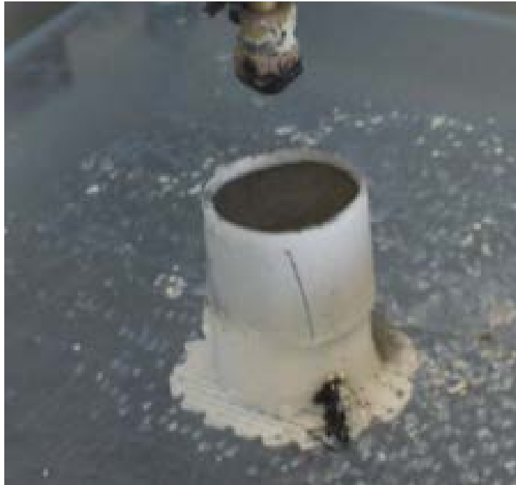
Figure 7.2: Additive Manufacturing of a battery cell: Showing a partial built, with a partially extruded thermo-polymer based case, and a fill of manganese oxide paste.
