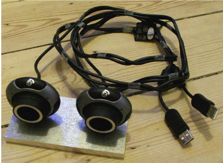
Figure 2.20: An experimental stereo camera system employing two high-resolution web cameras.
