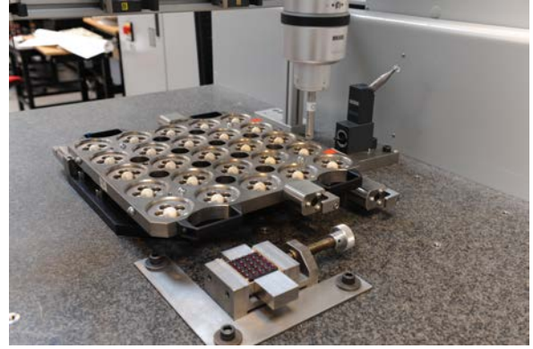
(b) CT ball plate during the traceability transfer.
