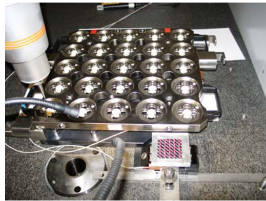
(b) CT ball plate during the traceability transfer.
