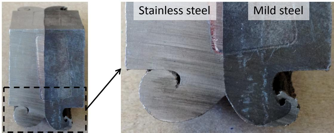
**Fig. 9.8.** Example of friction welded mild steel to stainless steel. The geometries of the formed flashes of the two materials are comparable to the shape of the material squeezed out during cross-wire welding.
