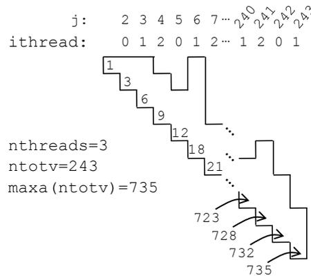
**Fig. 6.4.** Schematic skyline matrix with 243 degrees of freedom and a total skyline vector length 735. The example shows processing on three threads. The numbers in the diagonal correspond to the diagonal positions in the skyline vector. Numbers above the matrix show column number,  $j$ , and the thread number,  $ithread$ , of the thread to process a given column.
