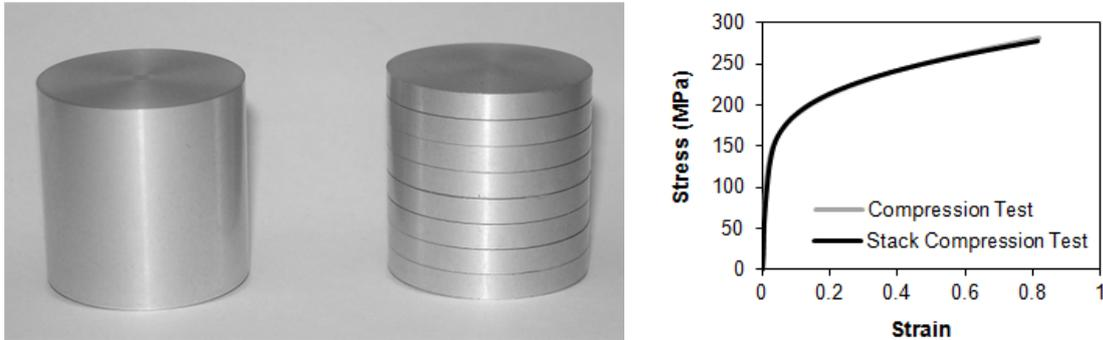
**Fig. 7.2.** Conventional and stack compression tests of Aluminum AA2011-O.
