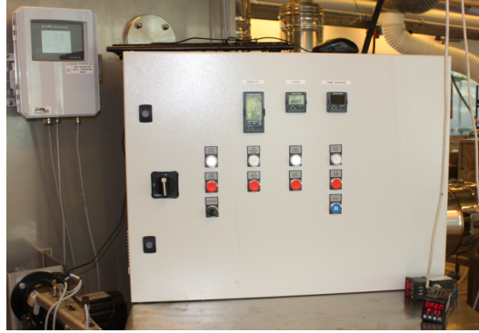
(b) Control panel, display on the humidity sensor and air duct trolley motor
