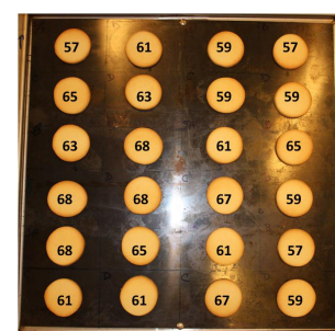
Figure 3. Calculated heat transfer coefficients (W/(m 2 K)), determined at the positions of the cookies baked to test the uniformity of browning.
