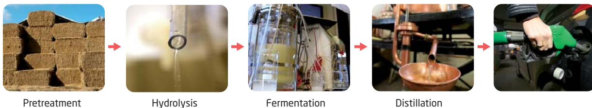
Fig. 8.6. Process steps for producing bioethanol from lignocellulosic biomass
