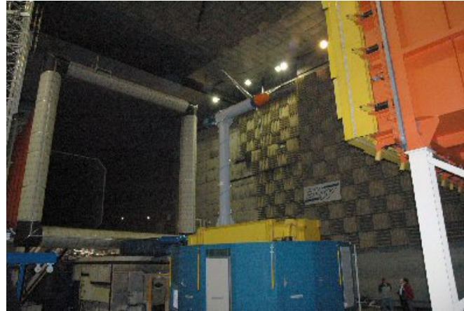
Model rotor tests "NREL Phase VI" (10m diameter) i NASA Ames 24mx36m testsektion
