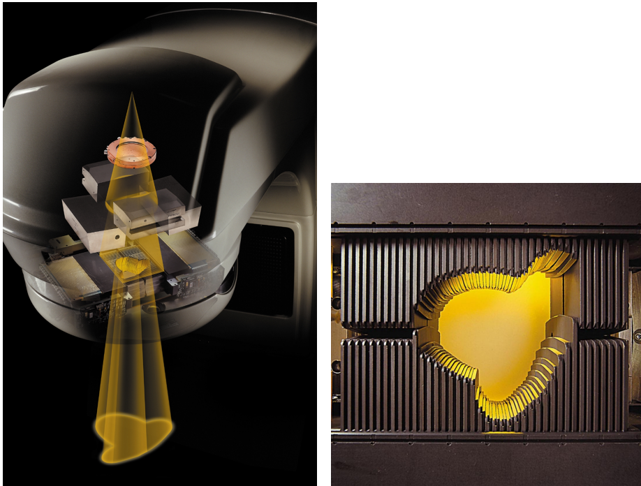
Figure 1.2: Left: An external beam radiotherapy device shaping the X-ray beam with a multileaf collimator (MLC). Right: Close-up of an MLC. Images courtesy of Varian Medical Systems, Inc. All rights reserved.
