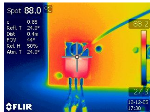
Fig. 10. Measurements when emissivity is \epsilon = 0.85 at the largest distance between components.
