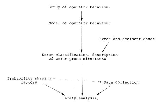
Fig. 1 Steps toward a detailed analysis of operator error.
