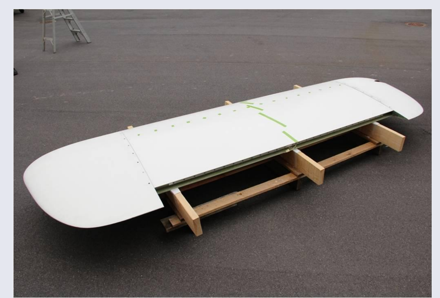
Blade section ready for mounting the flap
