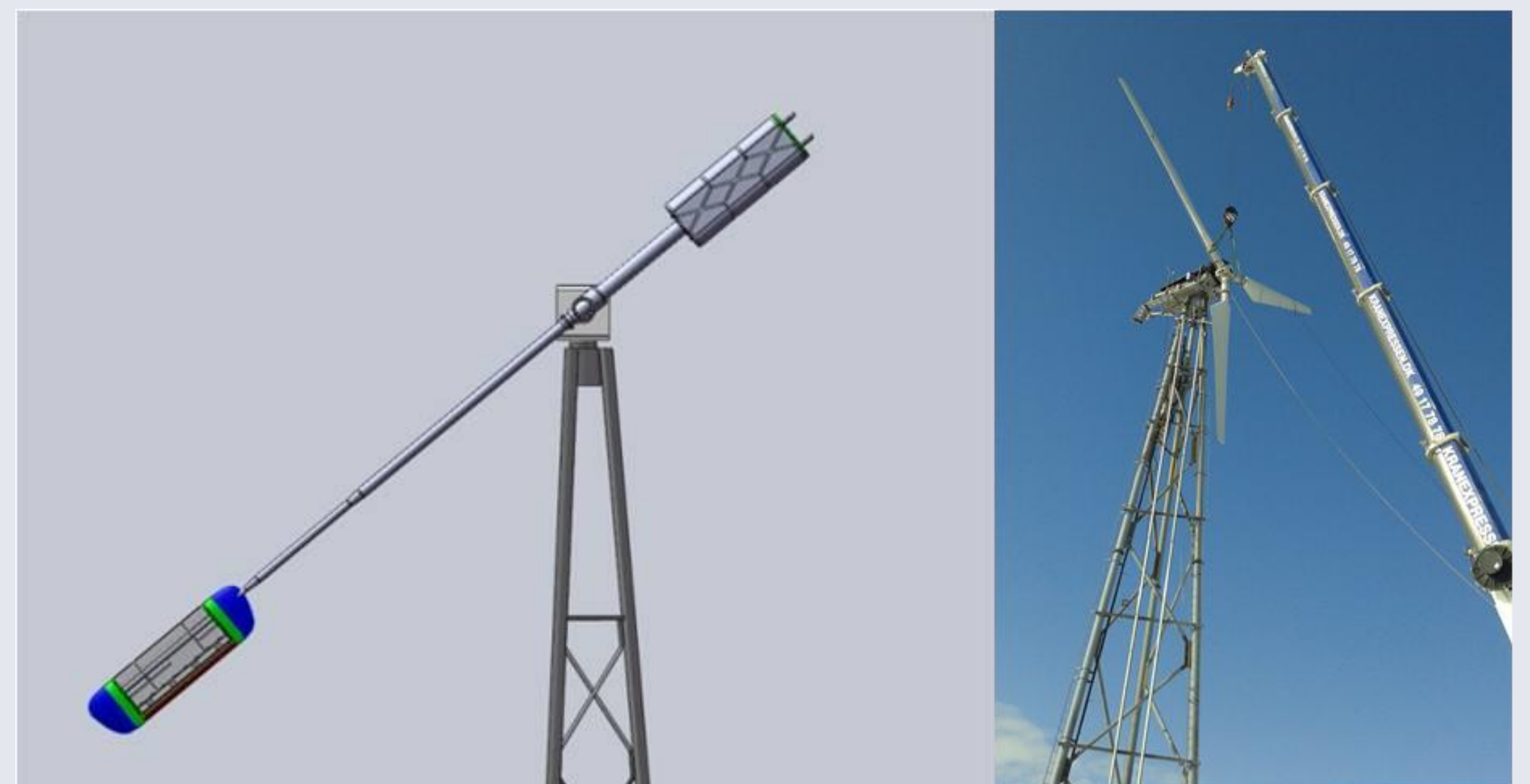
The rotating test rig is based on a 100kW turbine platform where a 10m long boom with the 2m x 1m blade section with flap is mounted instead of the normal three bladed rotor.
