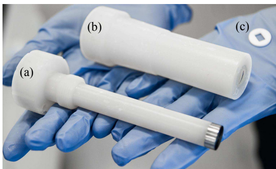
FIGURE 6.3: Custom-made sample holder used for electrochemical characterization of the anode in the three-electrode electrochemical set-up. (a) The stainless steel rod, (b) cover and (c) teflon mask.
