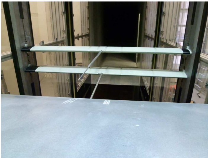
Figure 2. Slanted hot-wire holders set-up
