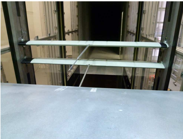
Figure 2. Slanted hot-wire holders set-up
